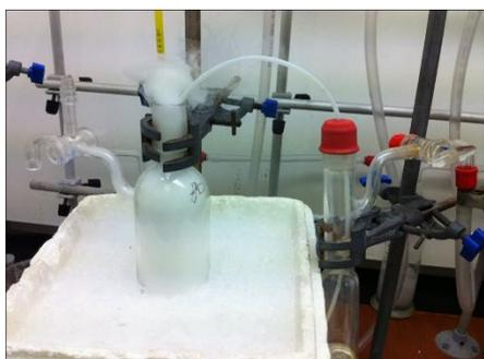
Figure 5-1: A photo of process of transferring titanium (IV) chloride (TiCl<sub>4</sub>) to a stable solution of titanium oxychloride (TiOCl<sub>2</sub>).
