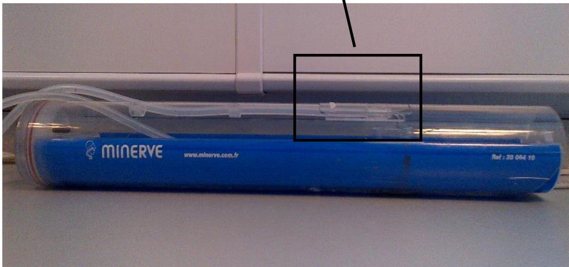
**Figure 4.22.** Modified Minerve small animal imaging bed
