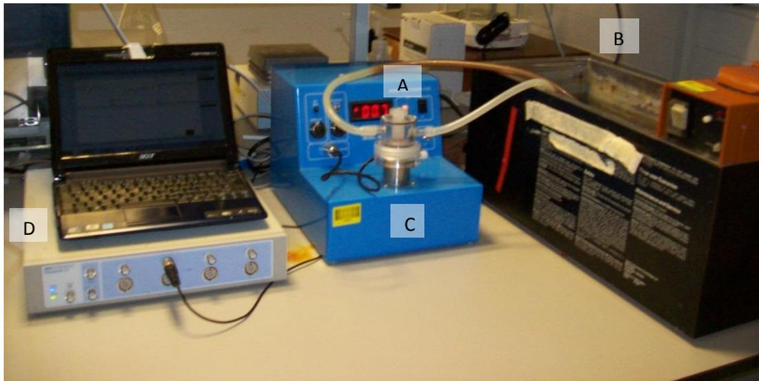
**Figure 2.5.** Experimental setup for mitochondrial respiratory measurements. (A) Isolated mitochondria were added to the electrode chamber and (B) maintained using a 30°C water bath. (C) Oxygen consumption was measured using a Clark-type oxygen electrode and (D) respiration rates recorded using a PowerLab system and chart5 software.
