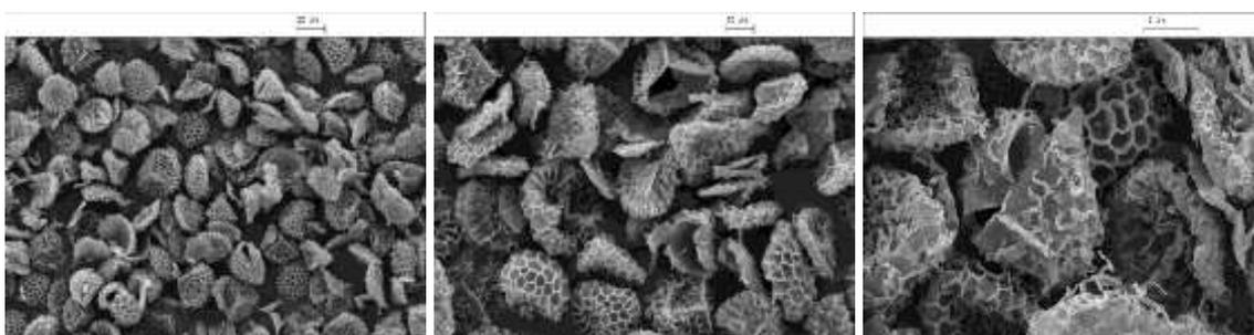
Figure 4.7 SEM images of BL-SECs following reaction with copper(II) nitrate solution. (The left-hand scale bar is 20  $\mu\text{m}$ , the central and right-hand ones are 10  $\mu\text{m}$ ).
