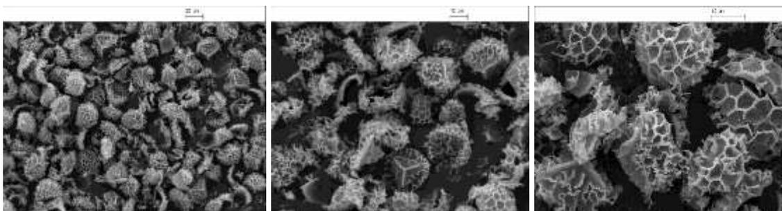
Figure 4.6 SEM images of BR-SECs following reaction with copper(II) chloride solution. (The left-hand scale bar is 20  $\mu\text{m}$ , the central and right-hand ones are 10  $\mu\text{m}$ ).
