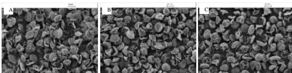
Figure 6.2 SEM images of BL-SECs after reaction with (A)  $\text{NiCl}_2$  solution, (B)  $\text{Ni}(\text{NO}_3)_2$  solution and (C)  $\text{Ni}(\text{OAc})_2$  solution.
