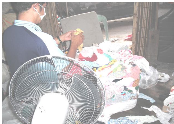
Figure 22 using fans to create draught for improving ventilation
