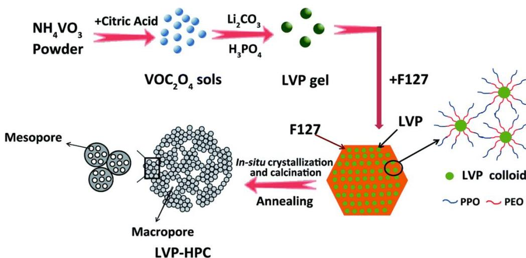
**Figure 1.8.** Schematic of the production of LVP-HPC. Reproduced from Y. Cheng, W. Zhou, K. Feng, H. Zhang, X. Li and H. Zhang, *RSC Adv.*, 2017, **7**, 38415–38423 – Published by the Royal Society of Chemistry. (Reference 64).
