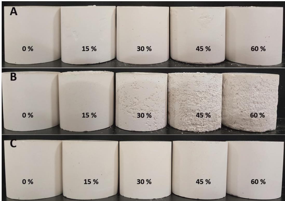
**Figure 3.2.** Photographs of the porous gypsum composites produced using different methods. (A) and (B) show the samples produced using small hydrogel beads and large hydrogel beads, respectively. (C) shows the composites produced using viscous trapping with the aqueous MC solution. The percentages on the images represent the volume of template used during their production.
