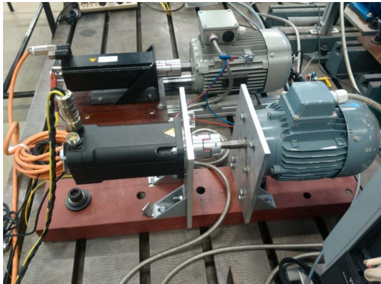
Figure 2-1 Induction motor driving systems (Chen et al., 2013)
