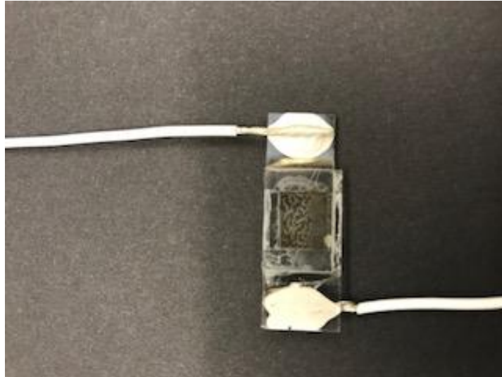
Figure 5-65: The cell of PDLC (5CB doped with chitosan) doped with SBB dye.
