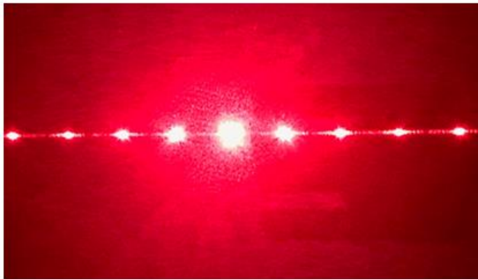
Figure 5-43: Far-field Fraunhofer diffraction pattern of the agarose relief grating, illuminated with a HeNe laser wavelength 632.8nm, 5mW.
