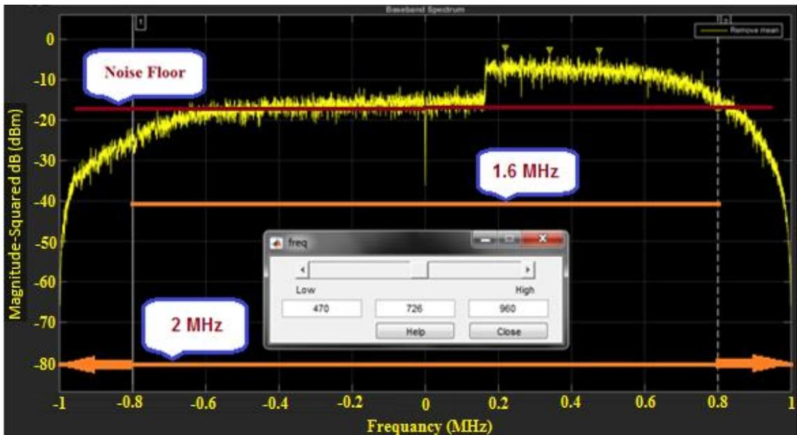
Figure 4-5: Measurement of centre frequency 726MHz in heavy raining day bandwidth 2 MHz
