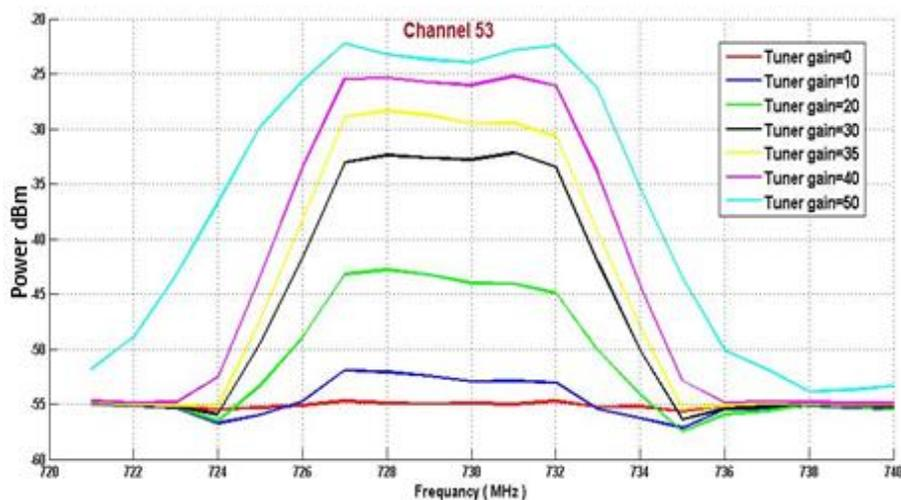
Figure 4-16: Average received power of channel 53 by different value of tuner gain
