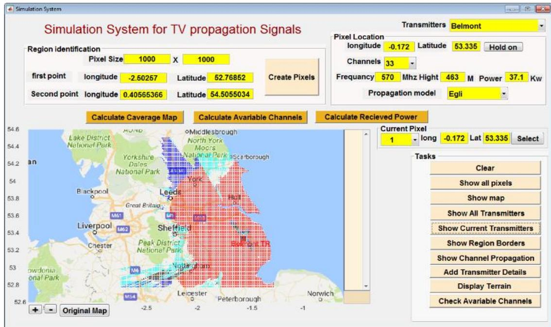
Figure 6-7: Display of the propagation signals for channel 33 using Egli model
