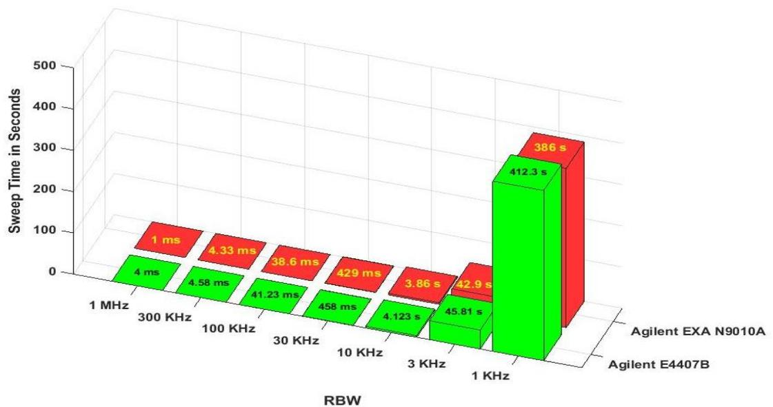
Figure 6-16: Sweep time of the Spectrum Analysers
