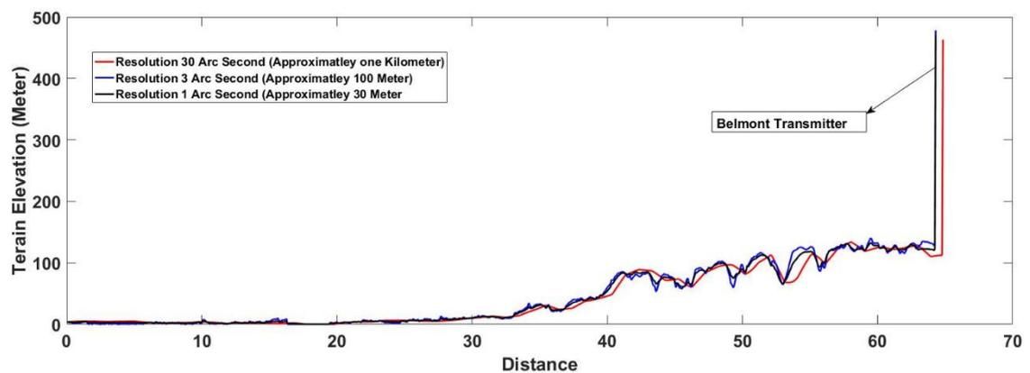
Figure 5-7: Terrain elevation data of the path from university of Hull to Belmont TV Transmitter in different resolutions.
