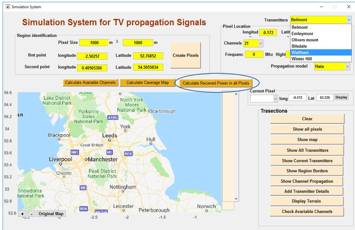
Figure 8.5: TV white space database system- Received power calculation
