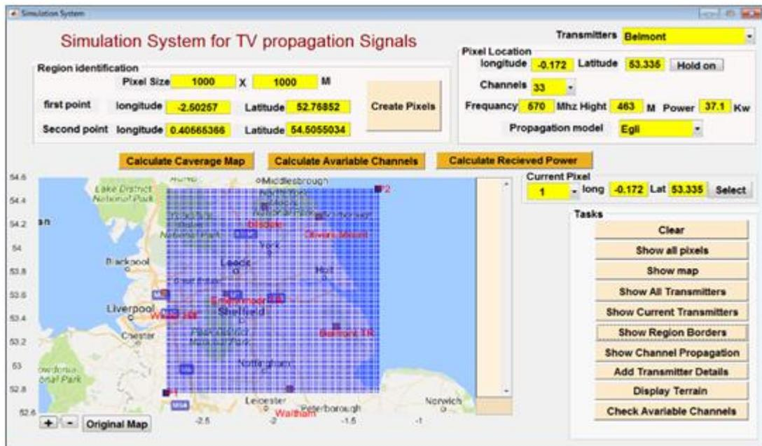
Figure 6-3: Display of all pixels in the selected region in the flexible simulation system for creating TVWS database
