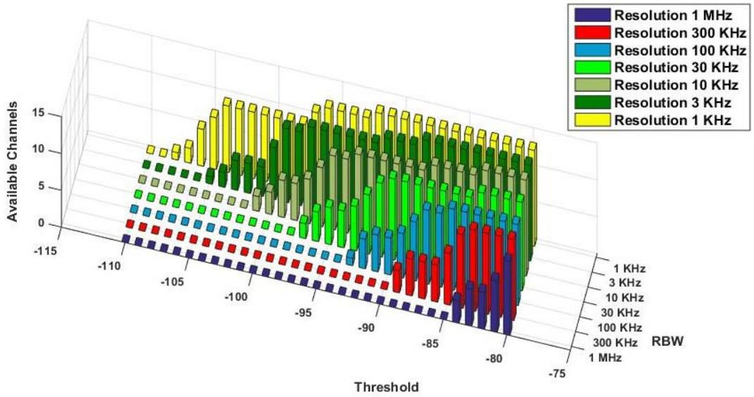
Figure 6-18: Calculation Thresholds, and RBW with Corresponding Available channels in spectrum Analyser EXA N9010A
