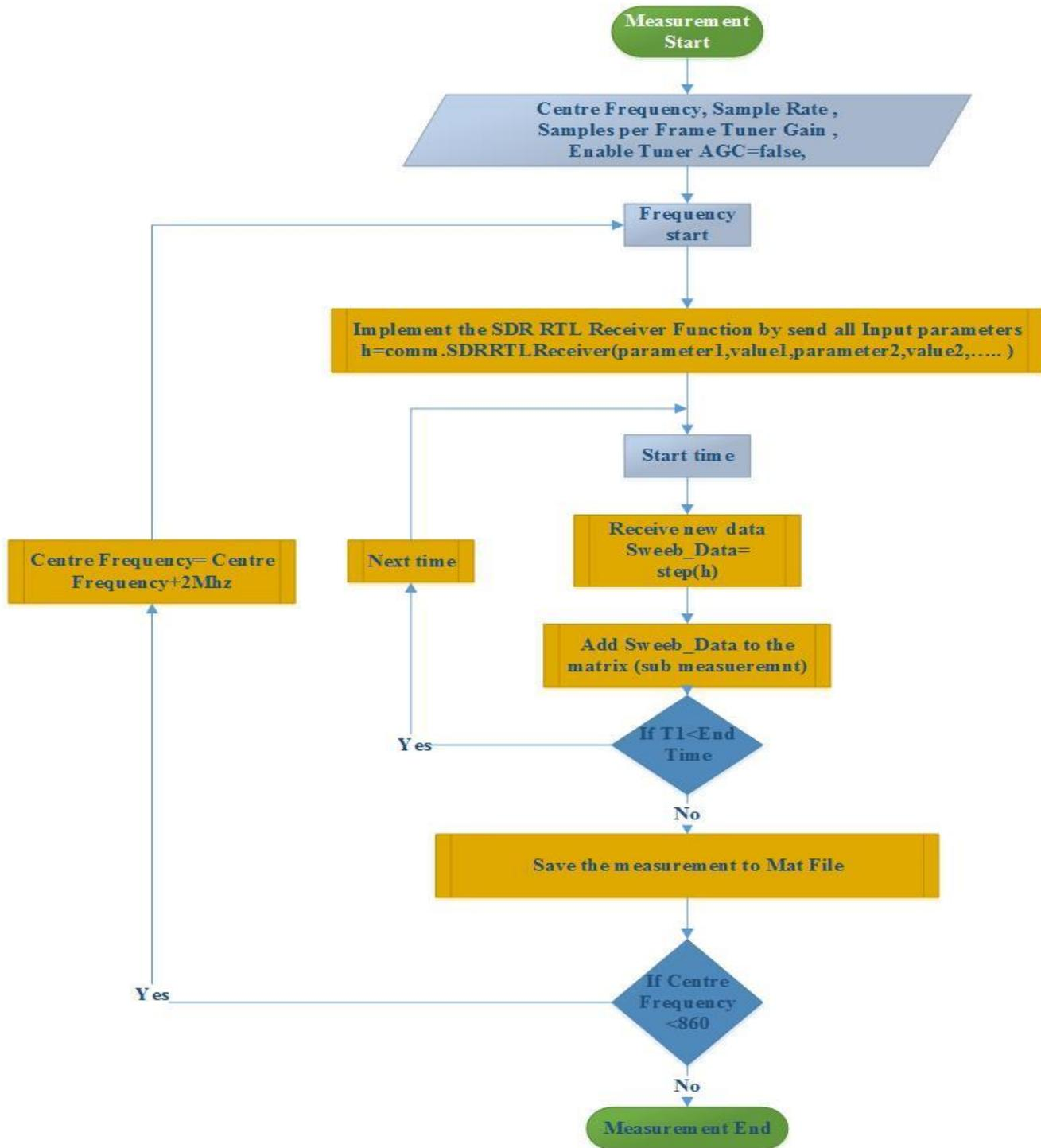
Figure 4-12: Signal calculation and Measurement methodology
