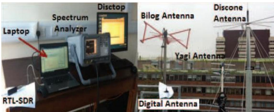
Figure 4-10: Measurement equipment in this paper: Antennas, spectrum analyser,
