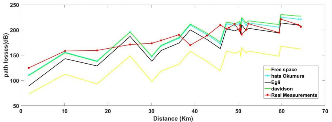
Figure 5-15: Propagation models included diffraction by using terrain profile with resolution 3 Arc second
