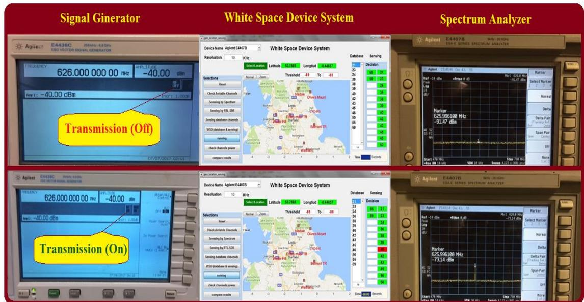
Figure 6-12: The white space system status before and after transmitting a test TV signal
