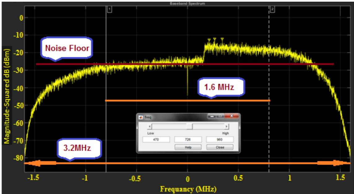
Figure 4-4: Measurement of centre frequency 726MHz in light raining day bandwidth 3.2 MHz
