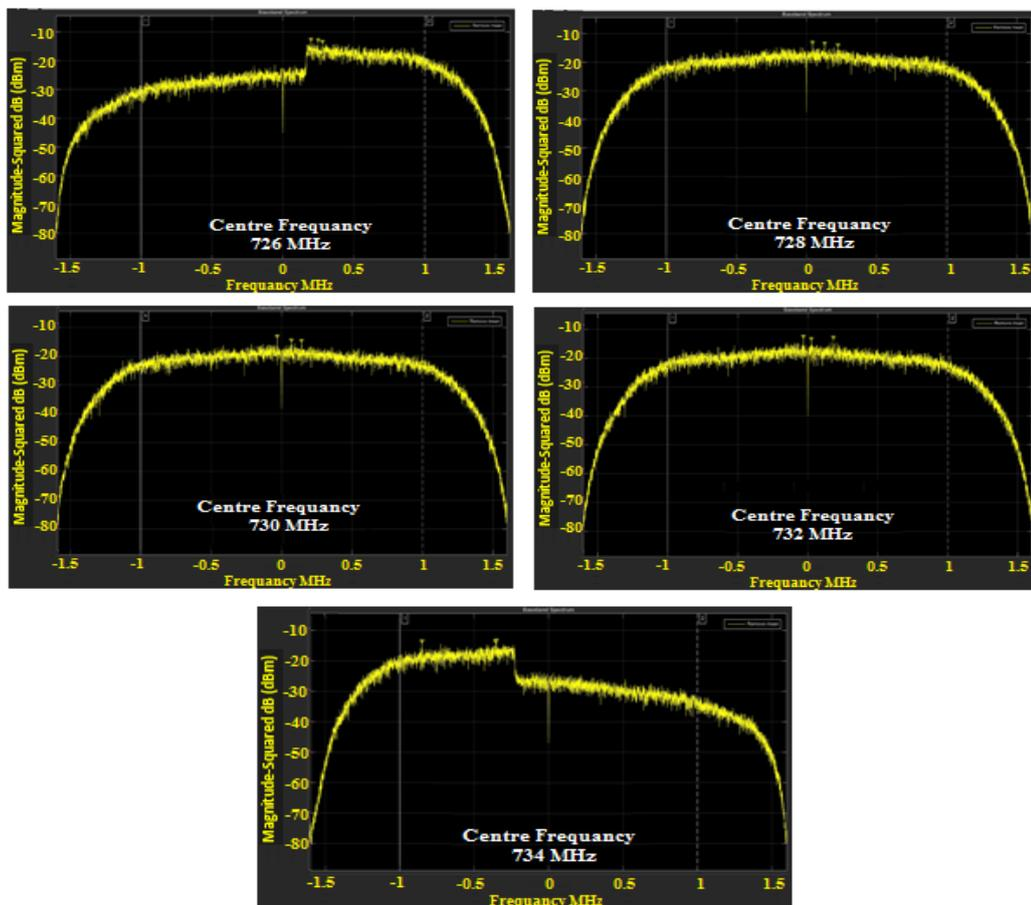
Figure 4-8: Channel 53 Measurement by using multiple hops technique
