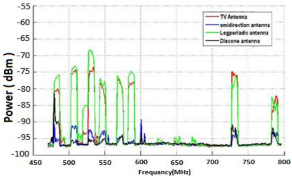
Figure 4-14: Average received power versus the frequency band 470-862 MHz by using RTL-SDR.
