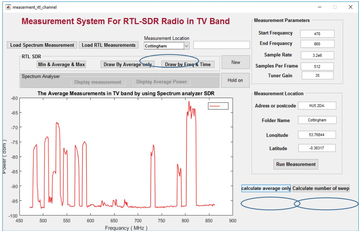
Figure 8.3: Measurement system - Display data Measurements
