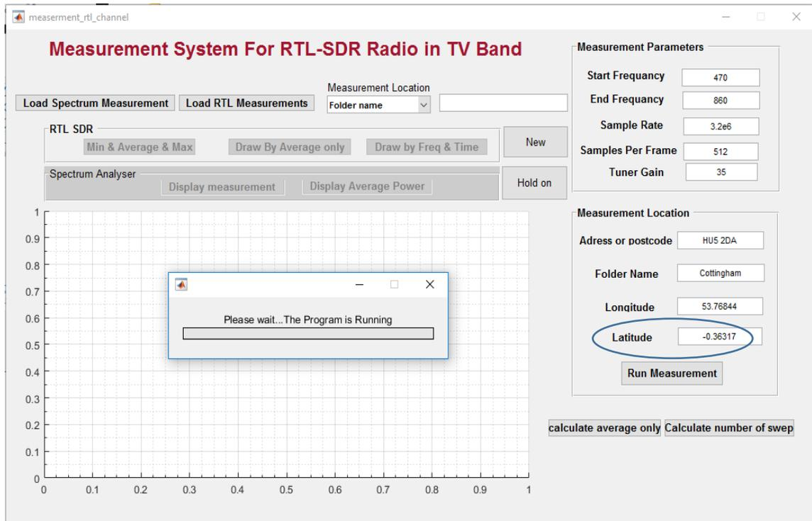
Figure 8.2: Measurement system - Measurement Implantation
