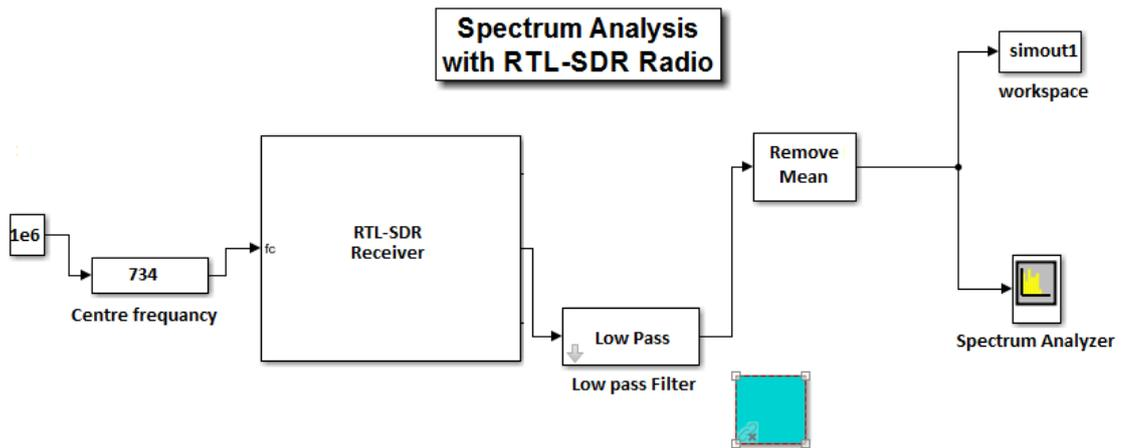
Figure 4-7: spectrum analysis with RTL-SDR radio Simulink diagram
