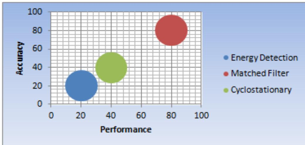
Figure 3-6: Comparison of spectrum sensing techniques (Singh, 2012a)
