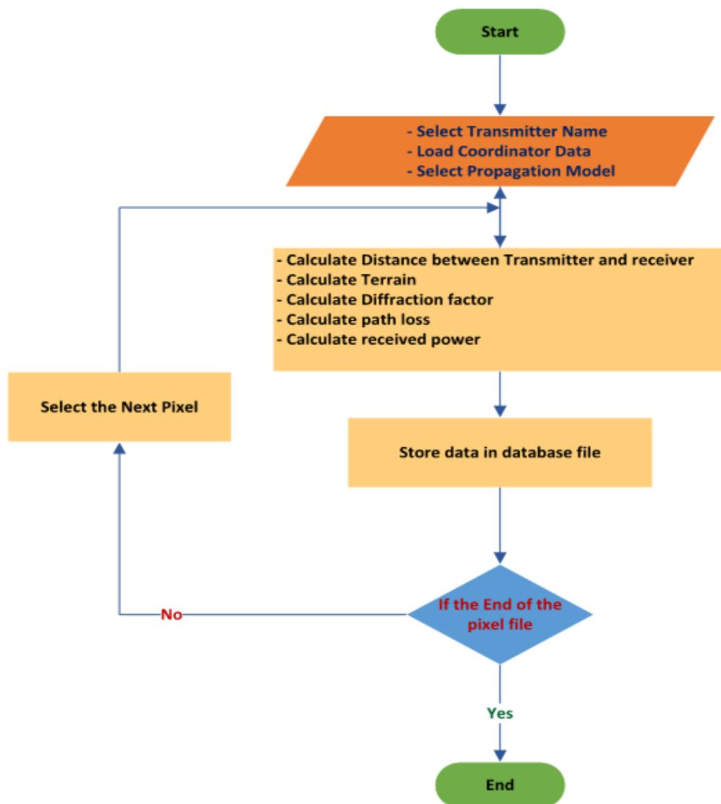
Figure 6-5 Algorithm of the received power calculation
