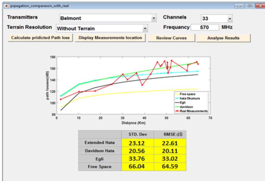
Figure 5-11: Example of propagation model comparison in the selected measurement locations
