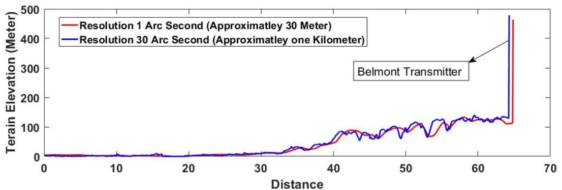
Figure 5-5: Terrain Elevation Data of path from university of Hull to Belmont Transmitter in different resolutions
