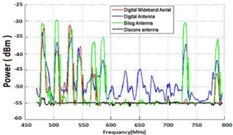
Figure 4-15: Average received power versus the frequency Band 470-862 MHz by using spectrum analyser.
