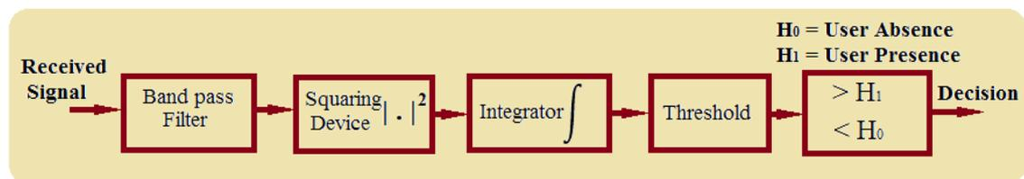
Figure 3-2: Energy detector block diagram
