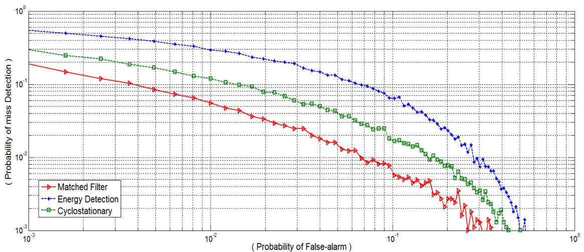
Figure 3-8: Complementary ROC curves for various spectrum sensing techniques (ED, MFD, CFD) with SNR=6 dB
