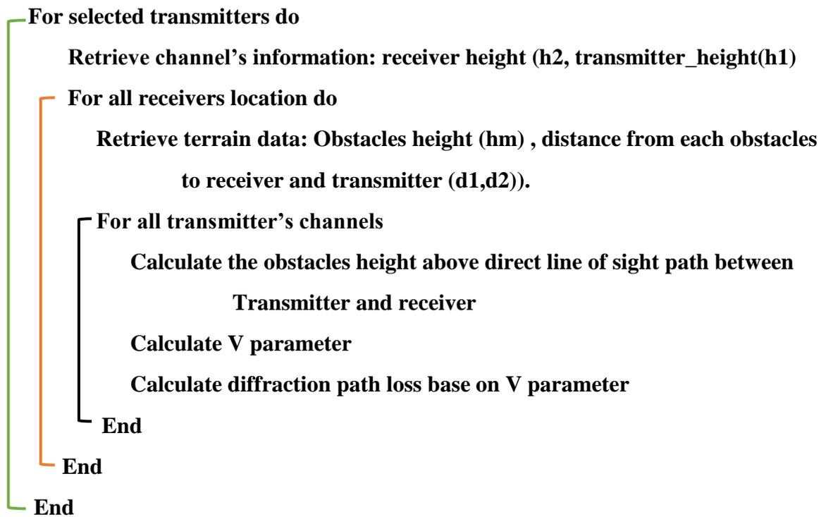
Figure 5-10: Algorithm of Diffraction Calculation
