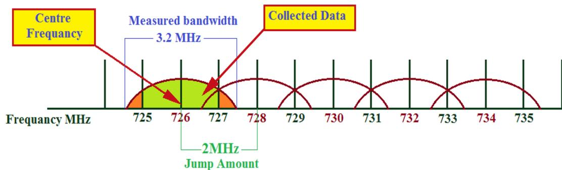
Figure 4-6: RTL-SDR Measurement Technique
