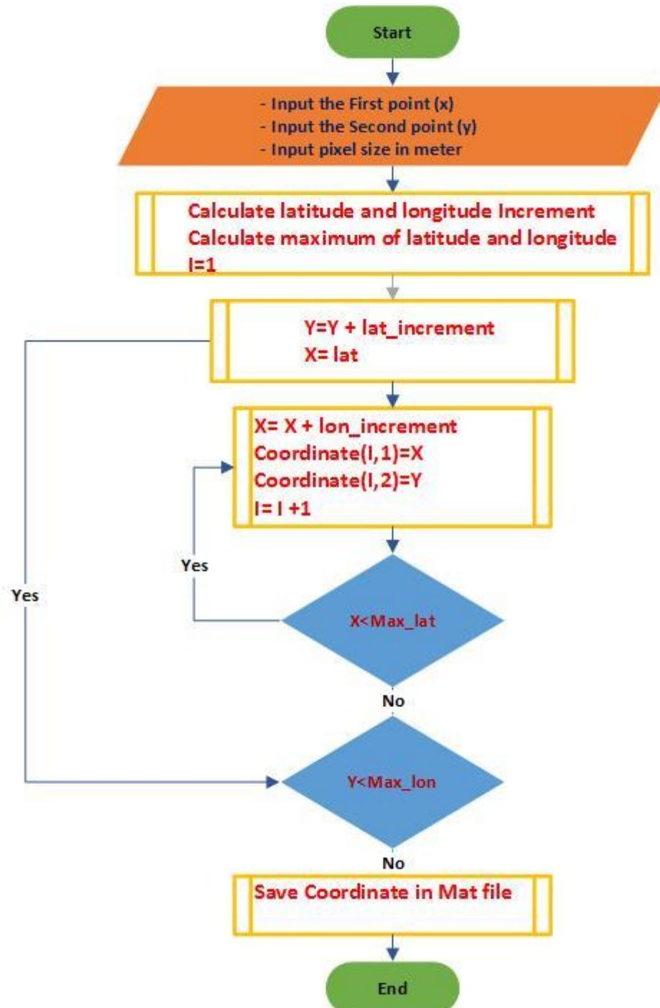
Figure 6-4: Algorithm of the Pixels Calculation
