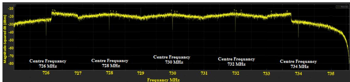
Figure 4-9: Channel 53 after combined the Measurement segments frequency range 726 MHz to 734 MHz
