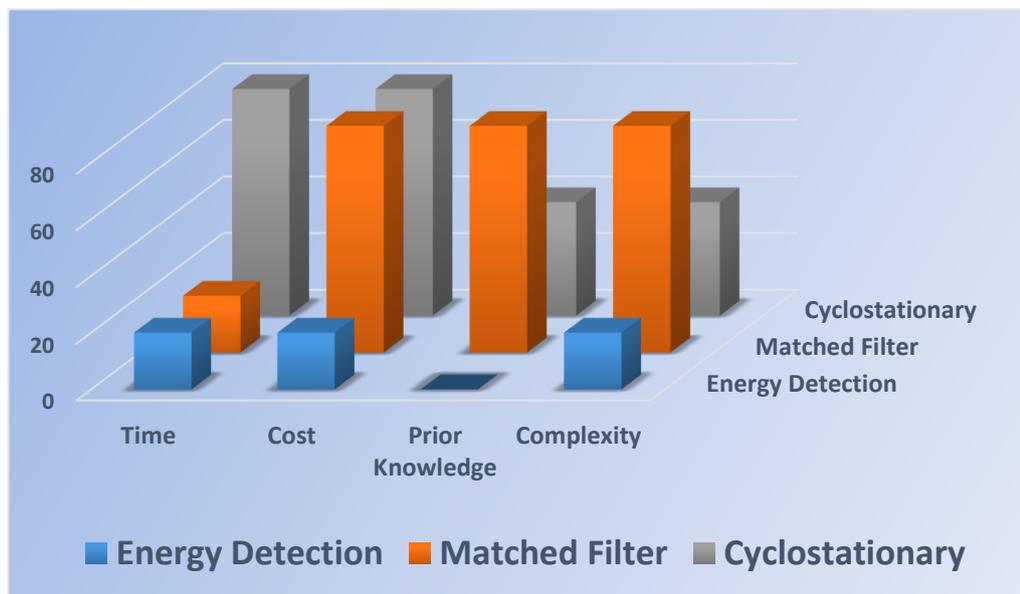
Figure 3-5: Comparison of spectrum sensing techniques
