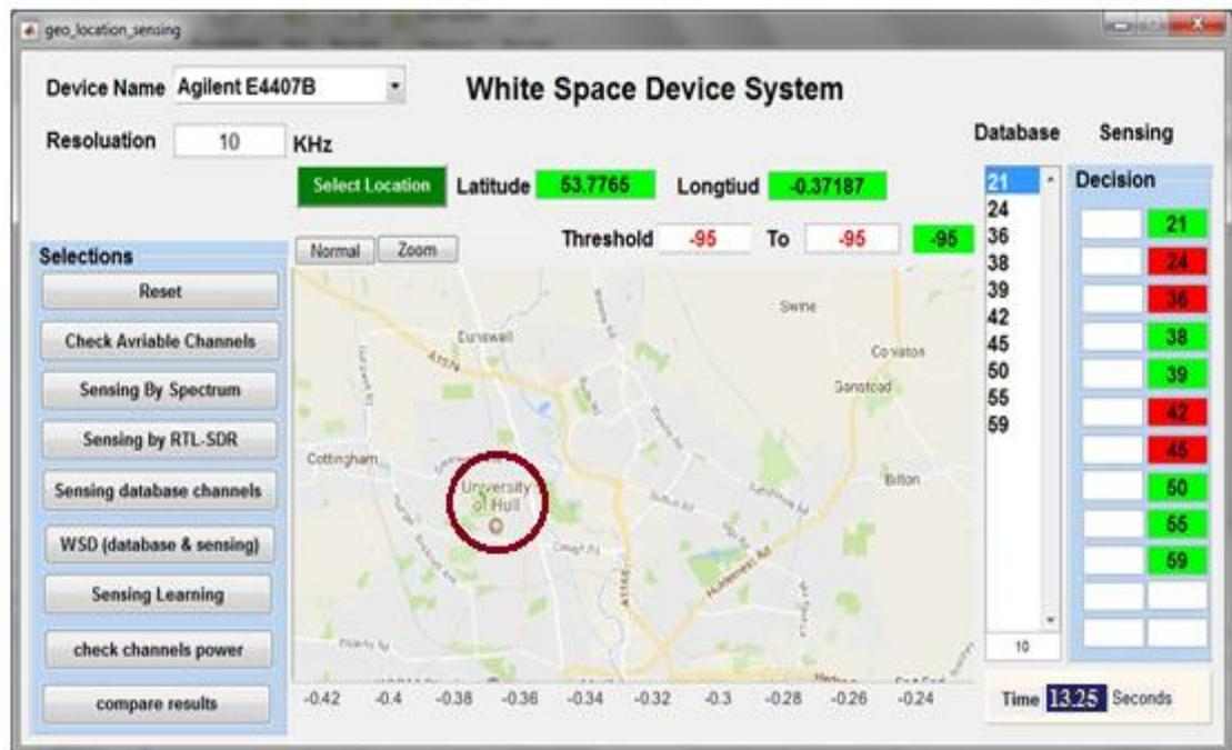
Figure 6-15: Results of combining techniques by using Agilent E4407B for sensing only database channels
