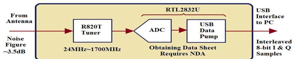
Figure 4-1: The RTL-SDR high level block diagram
