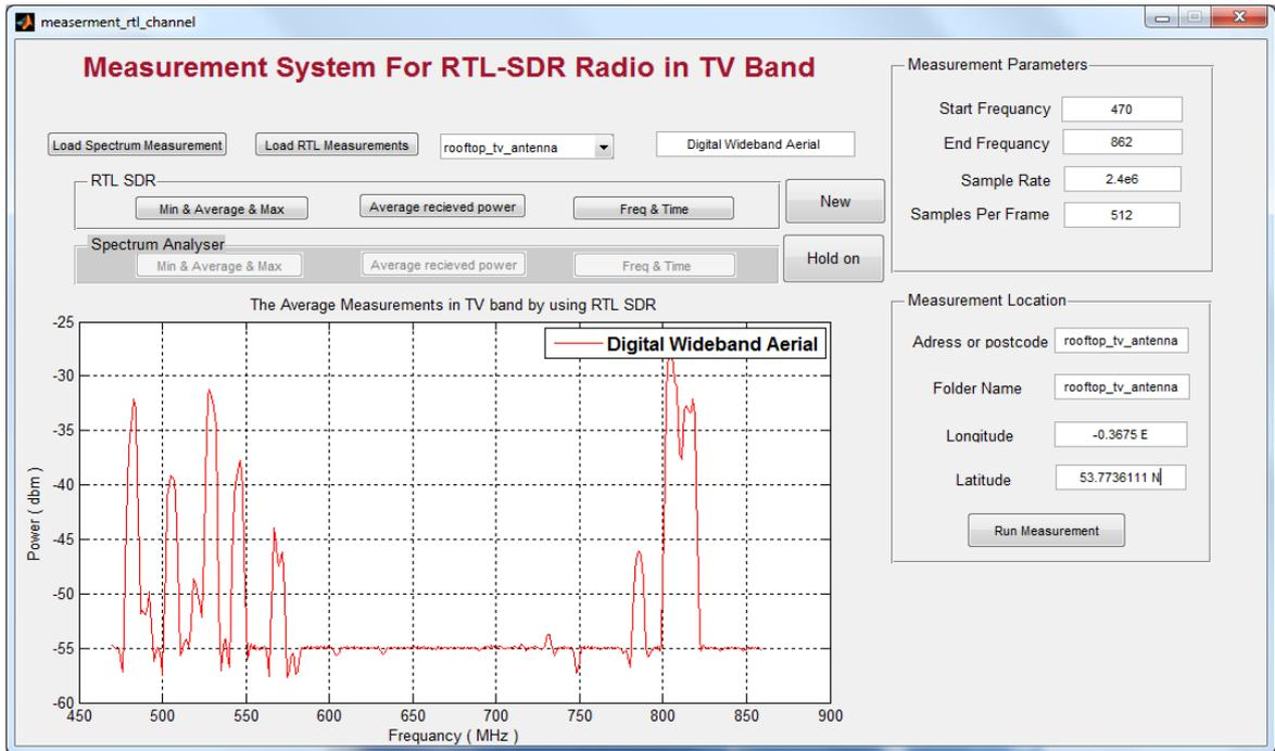
Figure 4-11: The GUI for the RTL-SDR System
