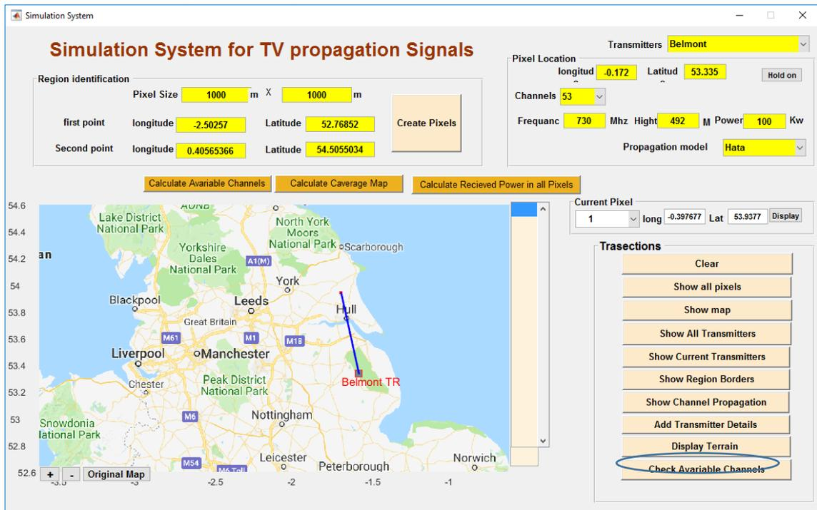
Figure 8.9: TV white space database system- Display the path from university of hull to Belmont transmitter
