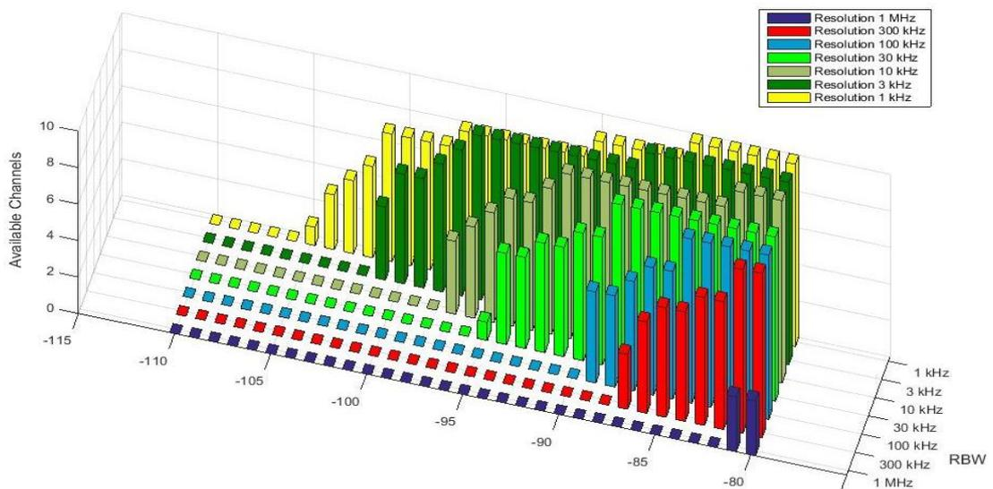
Figure 6-17: Calculation Thresholds, and RBW with Corresponding Available channels in spectrum Analyser E4407B.
