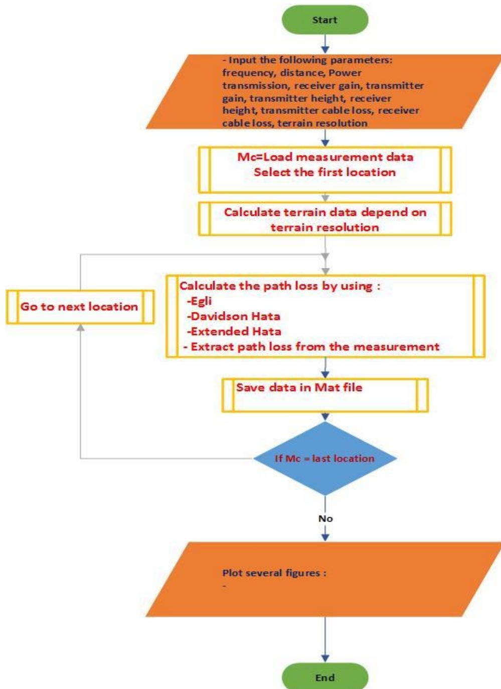
Figure 8.11: Comparison of propagation models algorithm
