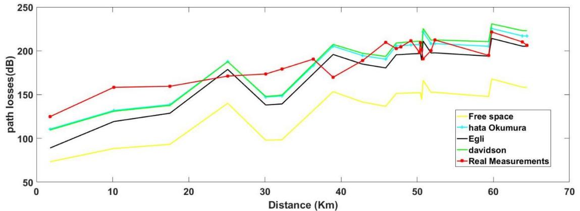
Figure 5-13: Propagation Models Including Diffraction by using Terrain Profile with Resolution 30 Arc Second (1 Km).
