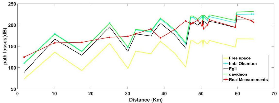
Figure 5-14: Propagation Models Included Diffraction by using Terrain Profile with Resolution 1 Arc Second
