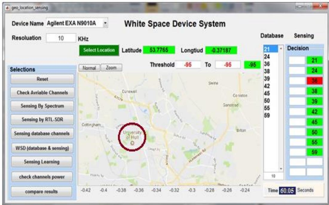
Figure 6-14: Result of combining techniques by using Agilent EXA N9010A with threshold
