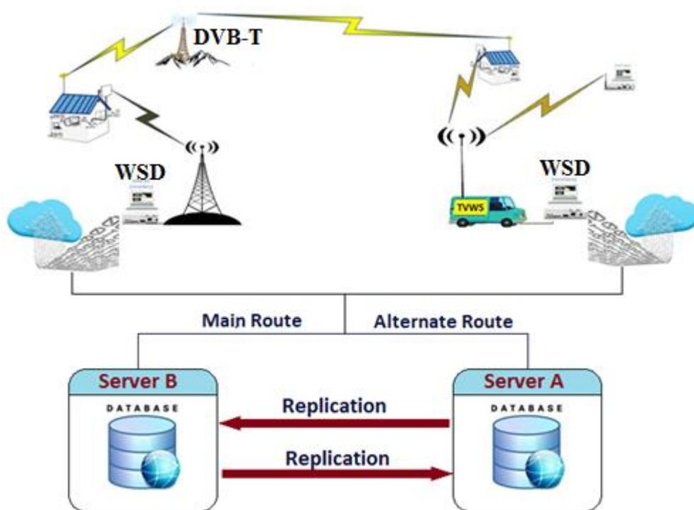
Figure 2-4: TVWS and Geolocation database mechanism
