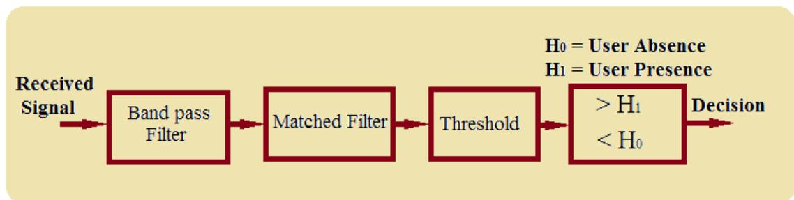
Figure 3-4: Matched Filter Detection block diagram
