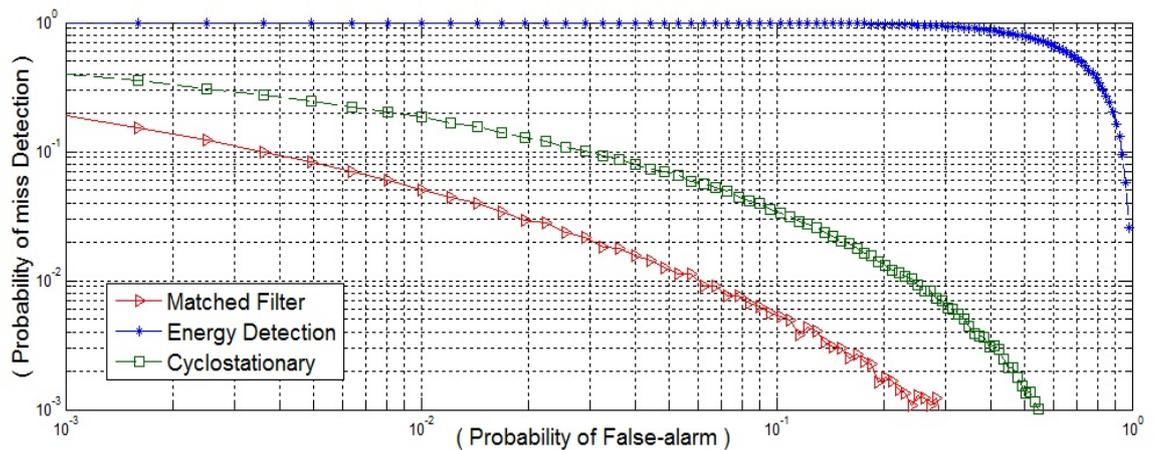
Figure 3-7: Complementary ROC curves for various spectrum sensing techniques (ED, MFD, CFD) with SNR=0 dB
