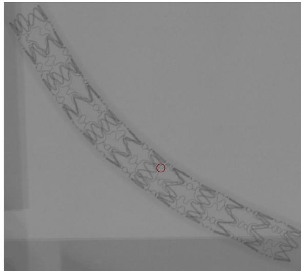
**Figure 5.8: Single fracture observed in Cypher stent deployed in silastic tubing of wall thickness 0.45 mm, after 552,257 cycles.**
