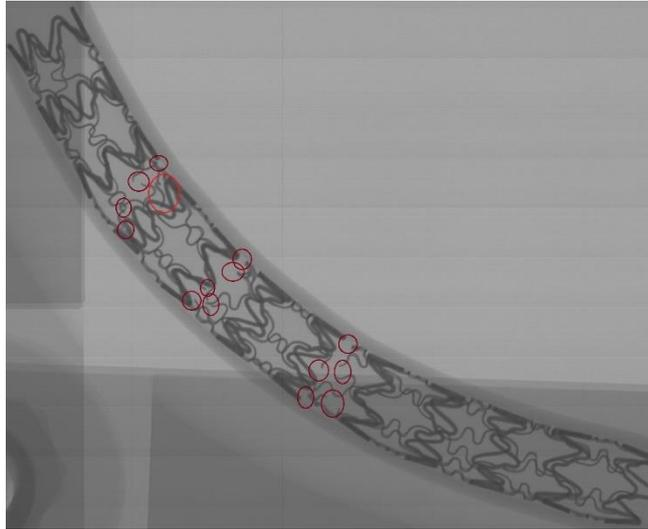
**Figure 5.9: 16 fractures observed in Cypher stent deployed in silastic tubing of wall thickness 0.45 mm, after approx. 4.2 million cycles.**
