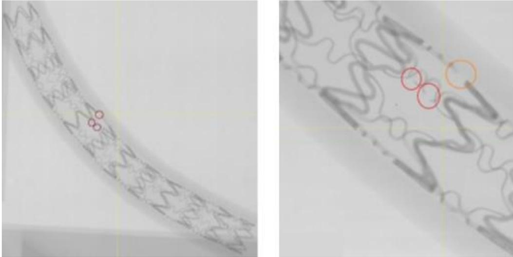
**Figure 5.7: Fractures observed in Cypher stent deployed in silastic tubing of wall thickness 0.75 mm, after 552,257 cycles.**
