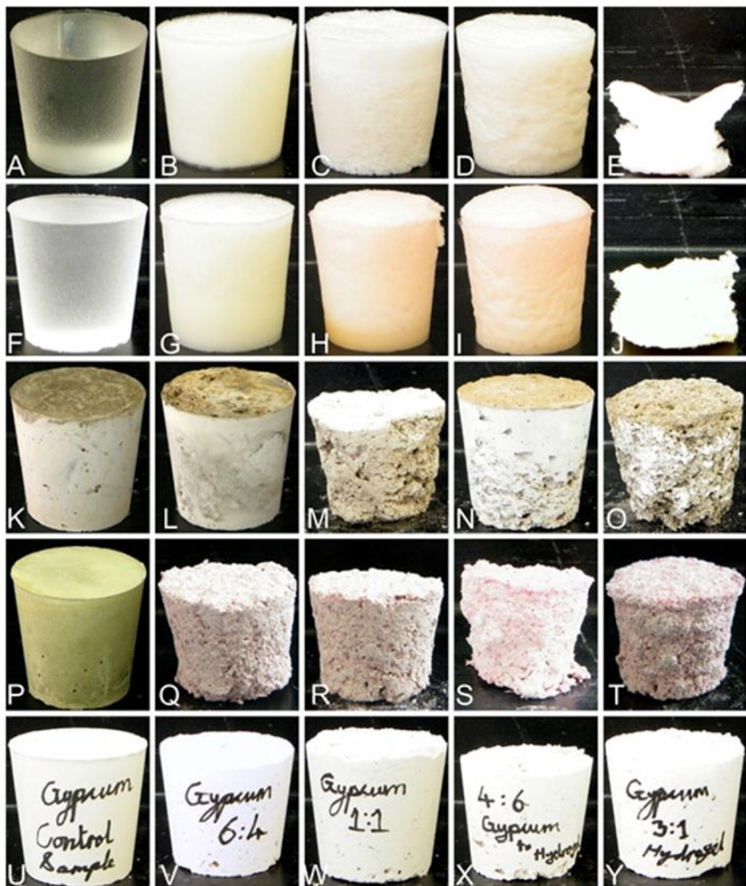
Figure 3.2. Moulded samples of:(A-E) PDMS with no silicone oil or surfactant, (A) control, (B) 50% gel, (C) 70%, (D) 80%, (E) 90%; (F-J) PDMS with surfactant and oil, (F) control, (G) 50%, (H) 60%, (I) 80%, (J) 90%; (K-O) cement: (K) control, (L) 66% hydrogel of 3 wt% gelling agent (M) 90% hydrogel of 3 wt% gelling agent, (N) 66% of 5 wt% gelling agent hydrogel, (O) 90% of 5 wt% gelling agent hydrogel; (P-T) talc-cement composite: (P) control, (Q) 50%, (R) 60%, (S) 90%, (T) 95%; (U-Y) gypsum: (U) control, (V) 40% hydrogel, (W) 50% hydrogel, (X) 60% hydrogel, (Y) 75% hydrogel.
