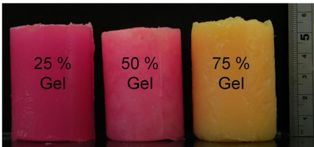
Figure 7.5. Image showing soap-hydrogel composites with a total 0.7 wt% of gelling agent (Xanthan : Konjac 2:1). Soap base was stained with Nile Red and the hydrogel with fluorescein sodium salt.
