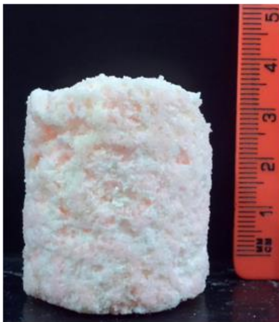
Figure 5.21. A photograph of a sample that was dried in open air at room temperature after freezing the sample at -20\text{ }^{\circ}\text{C} . The fat base was stained with Nile red and the hydrogel (1.5 wt% gelling agent, 50 vol% of the composite) with Fluorescein sodium salt.
