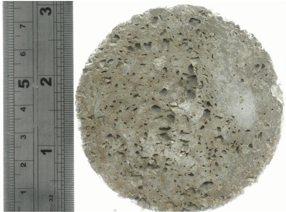
Figure 4.9. A photograph of the top of the sample of a porous cement sample (70 vol% hydrogel content) produced using 3 mm pore size mincer plate minced hydrogel. Sample diameter was 7.6 cm and thickness 2.0 cm designed to fit the sound impedance apparatus.
