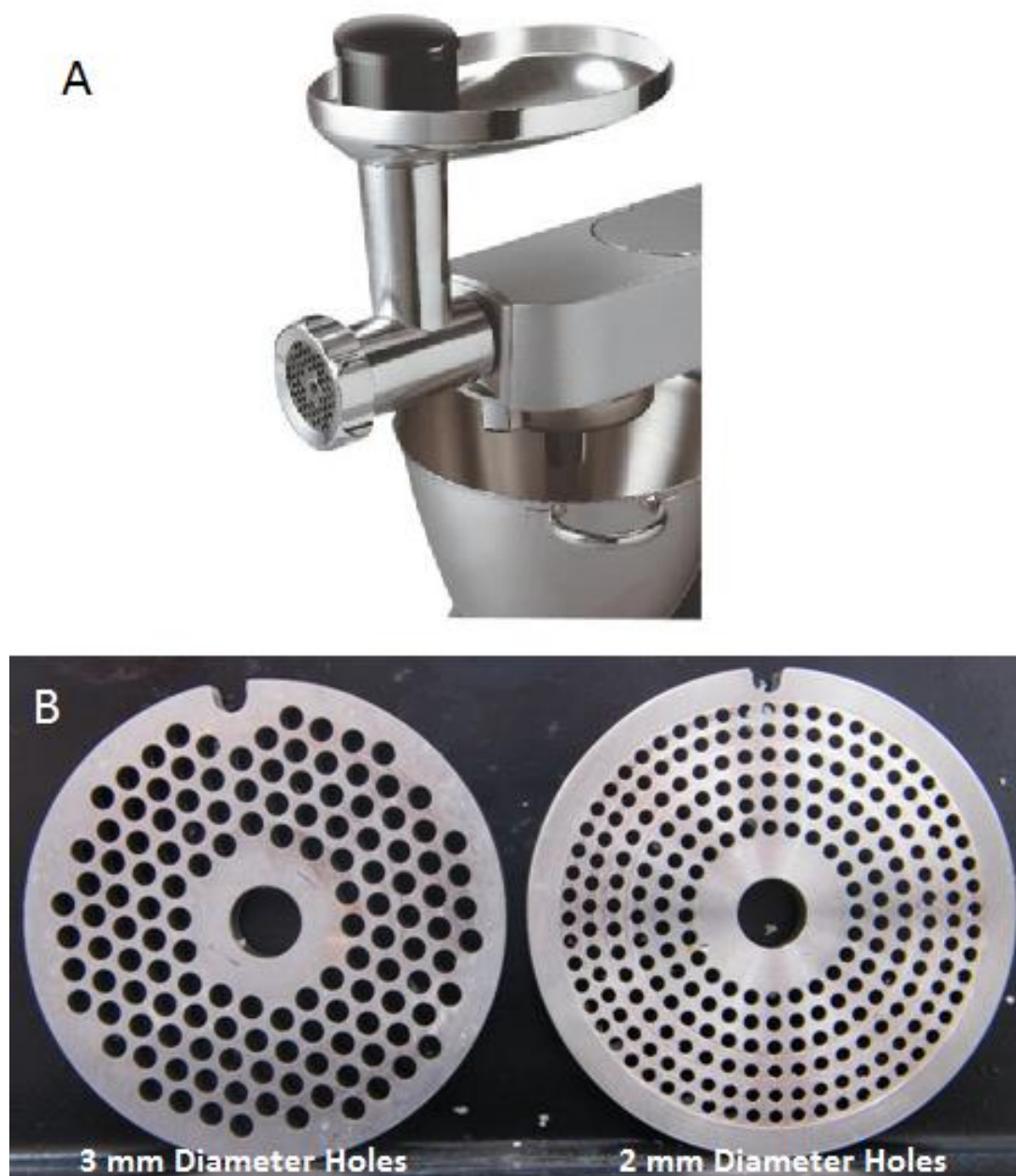
Figure 2.2. Images showing (A) Kenwood Chef mincing attachment used for the fabrication of hydrogel bead slurries, (B) the mincer plates with diameter 3 mm and 2 mm of the plate holes on the left and right respectively used to produce different bead size distributions within hydrogel slurries.
