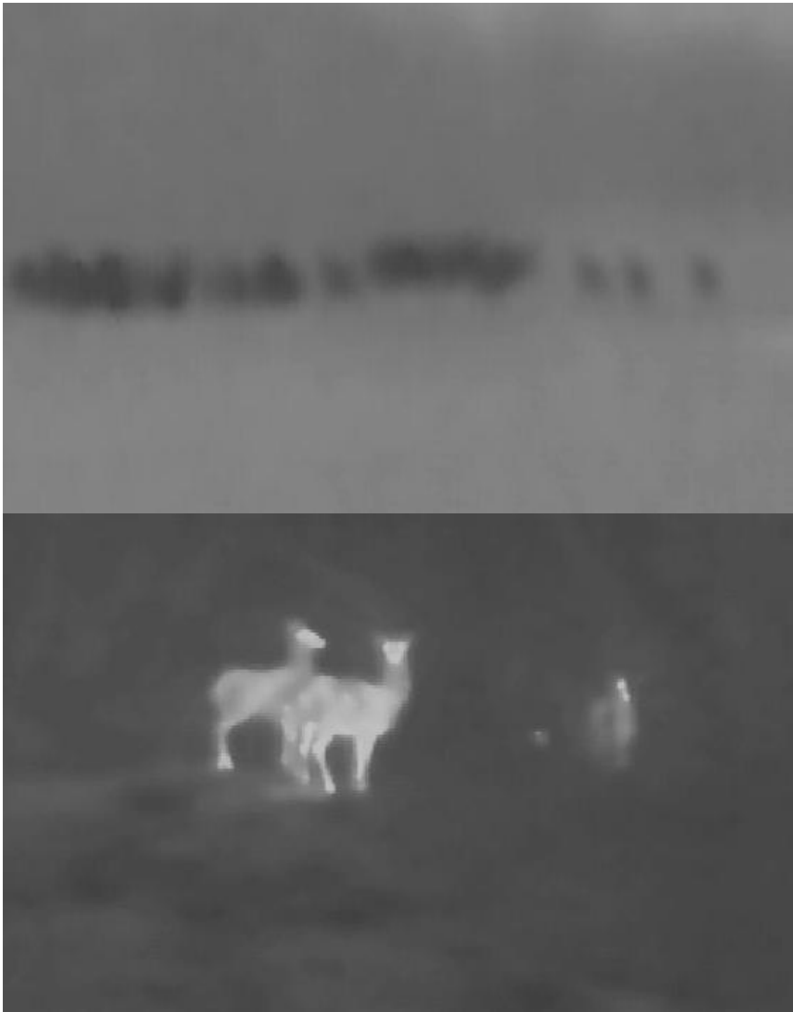
Figure 4.3. Two images of deer through the thermal imagers. The top image is a large herd of red deer at approximately 350-400m on a farmers field; using black as the hot indicator. The bottom image shows three red deer hinds approximately 40m away in dense vegetation; this image used white as the hot indicator. Photo credit: Thomas Logan, with permission.
