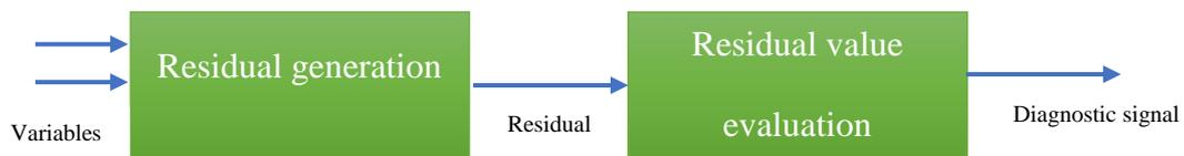
Figure 2.14 – Fault diagnostic diagram using residual generation
