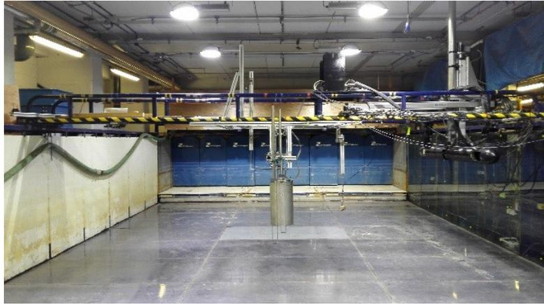
FIGURE 1.8: 1/50 scaled PAWEC and corresponding experimental wave tank at UoH (Jin et al., 2018).
