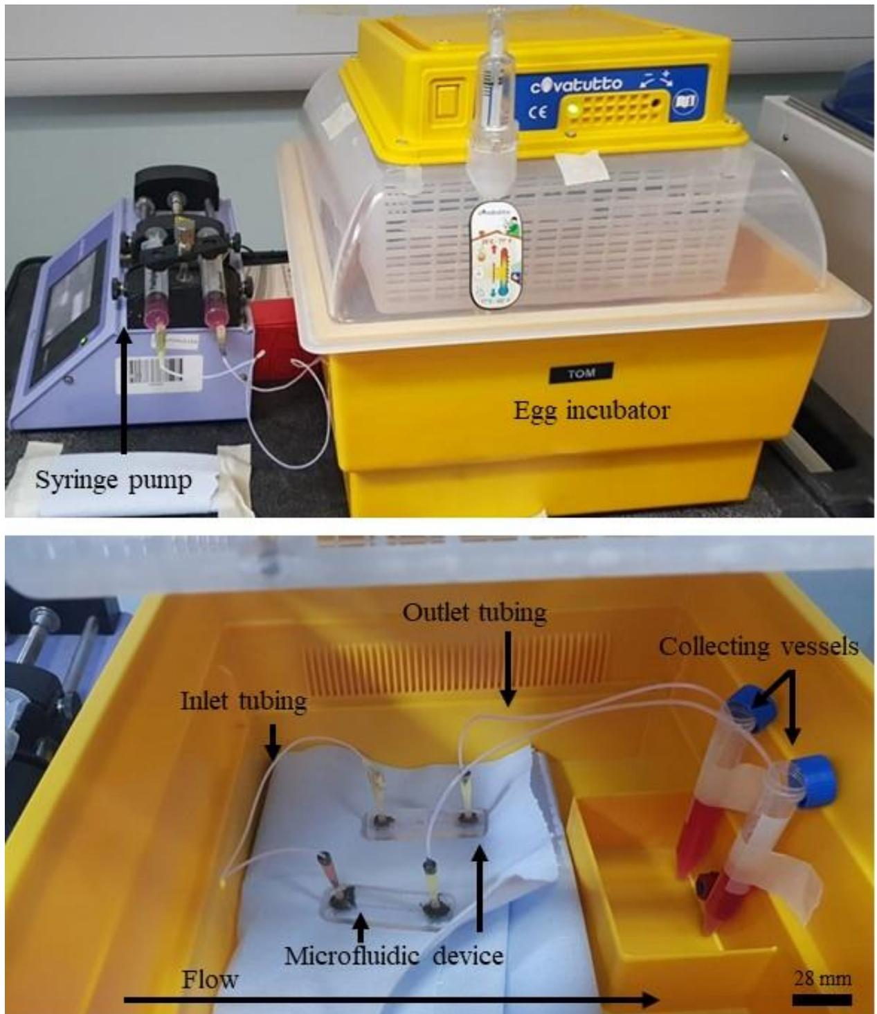
**Figure 4.4: Egg incubator and microfluidic device set up**
