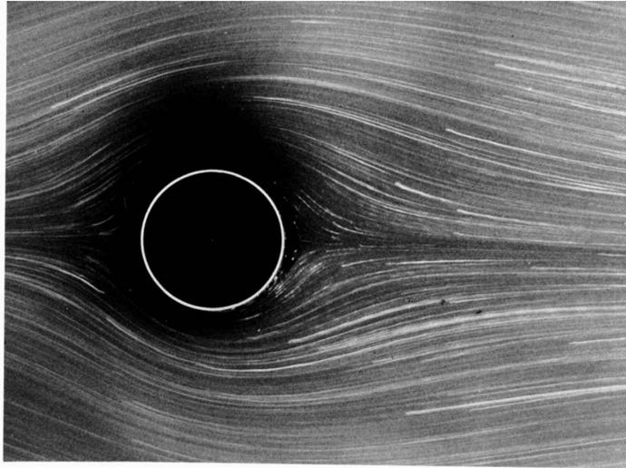
**Fig. A.1:** Taken from *The Album of Fluid Motion* by van Dyke & White (1982), Fig. 24, photographed by Sadatoshi Taneda. An example of Laminar flow around a sphere at a Reynold's number of 1.54. The flow shows the smoothness of the streamlines around the sphere characteristic of laminar flow.
