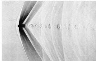
**Fig. 2.4:** Simulation run with the FLASH code of a Mach 3 wind flowing around a rigid rectangular domain at  $t = 0.0$  s,  $t = 200.3$  ms,  $t = 400.2$  ms,  $t = 700.2$  ms,  $t = 1.5$  s and  $t = 4.0$  s. The colours code the gas density. An image of a supersonic rifle bullet moving through air from van Dyke & White (1982) is also included to show the clearly similarities in the wave patterns, particularly the morphology of the shock waves.
