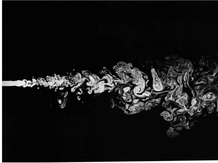
**Fig. A.2:** Taken from Dimotakis et al. (1983). Turbulent Flow from a water jet with Reynold's number  $\sim 2300$  revealing the formation and decaying of eddies.
