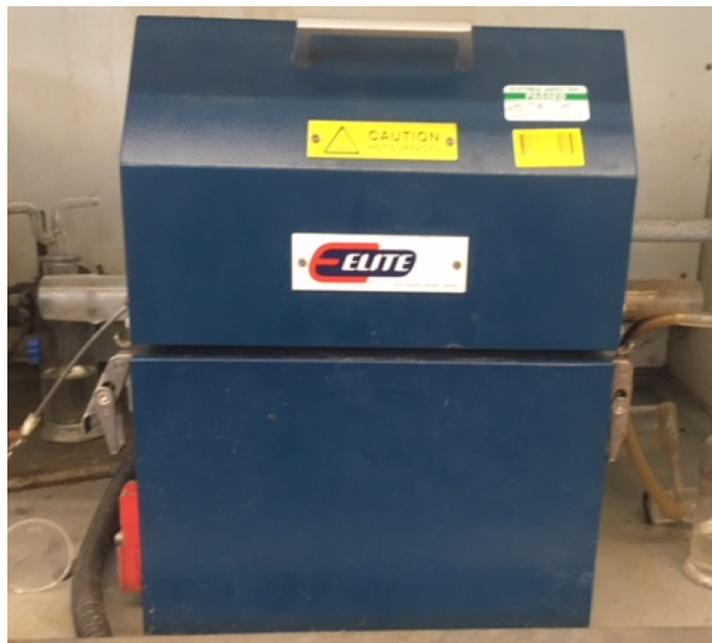
Figure 2.3: Elite thermal systems horizontal tubular furnace with quartz tube inserted.
