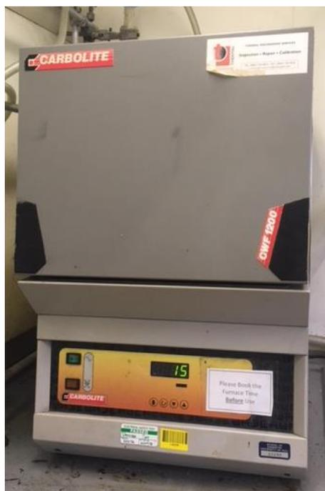
Figure 2.2: Carbolite CWF 1200 type box furnace.
