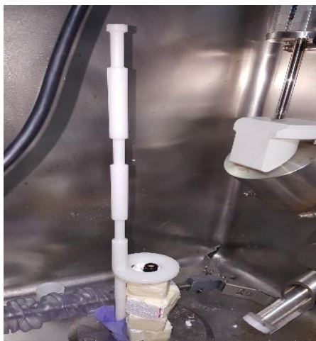
Fig 19: A vial containing certain amount of ^{18}\text{F} -FDG inserted within 1×1×1inch polystyrene box. The first measurement was taken with the vial touching the bottom of the capentec dose calibrator, subsequently the box was lifted by inserting another 1×1×1inch box beneath it until the vial containing box reaches the top of the calibrator
