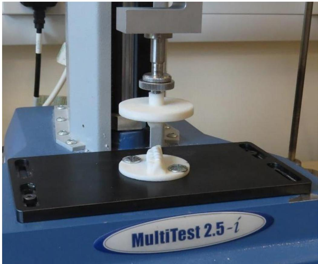
**Figure 2.18 Circular attachment plate prototypes attached to the universal materials tester.**
