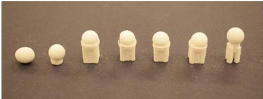
**Figure 2.24 Examples of supports for 10mm diameter spheres. The five supports and spheres to the right were created automatically by ZPrint Pro. The small support second from the left was designed by the author. On the far left is a “sphere” printed without a support.**
