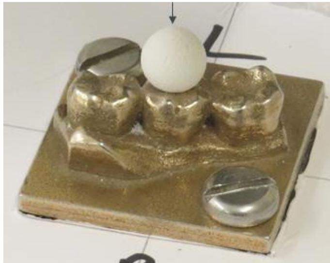
**Figure 3.4 Photograph of a sphere placed on the tooth model. The arrow indicates the pole used for alignment.**
