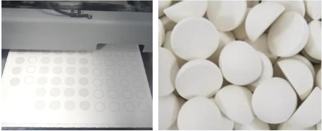
**Figure 2.13 3D printed domes (powder and binder) to be crushed in a sensitivity study of tooth design. (Images adapted from Swan 2016 and Hunter 2016)**
