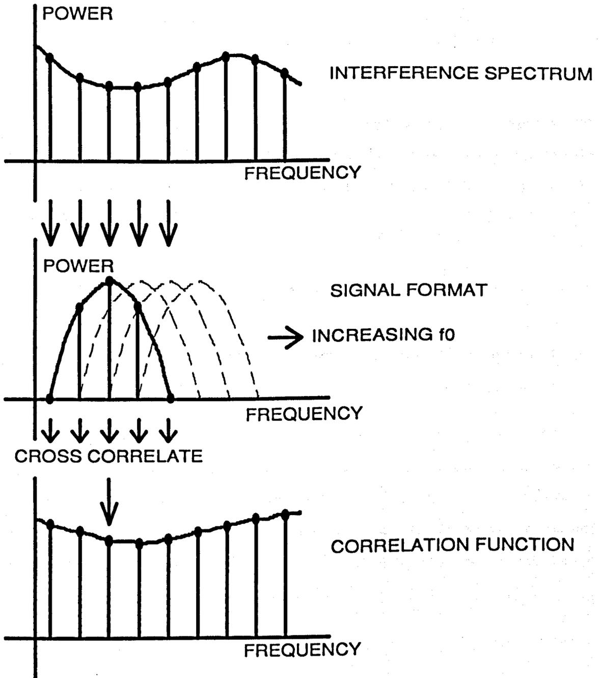
Hence, by performing the above frequency domain cross-correlation and then locating minima in the resulting correlation function, the points within a noisy channel that are most suitable for use by a particular modulation format are found.
