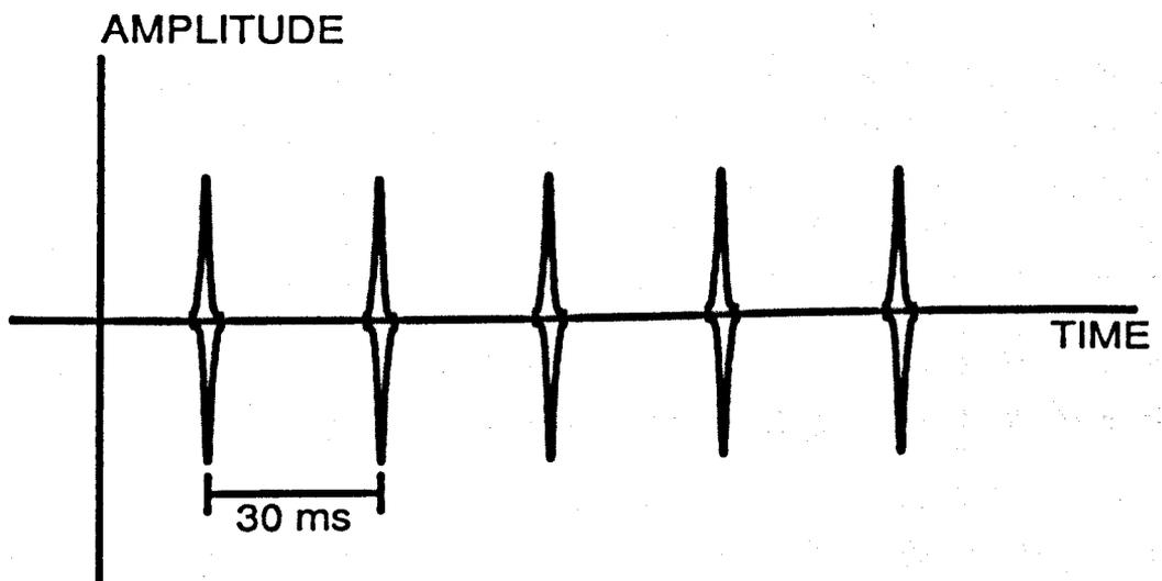
the same parameters as the chirps produced by the sounder transmitters would be more difficult to achieve in practice. The sample output rate and the number of samples were calculated so that a 30 ms portion of chirp waveform would be produced. This represents the length of chirp that would occur in a 3 kHz receiver bandwidth.
