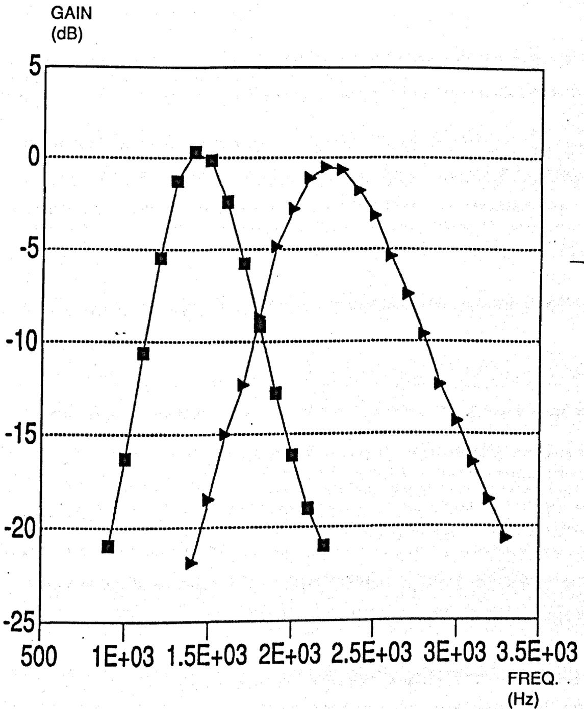
The demodulator filters were programmed to correspond to the tone frequencies of the Cossor demodulator and the bandwidth of each tone filter was set to be 100 Hz. The resulting filter amplitude response is shown by Figure 8.11.
