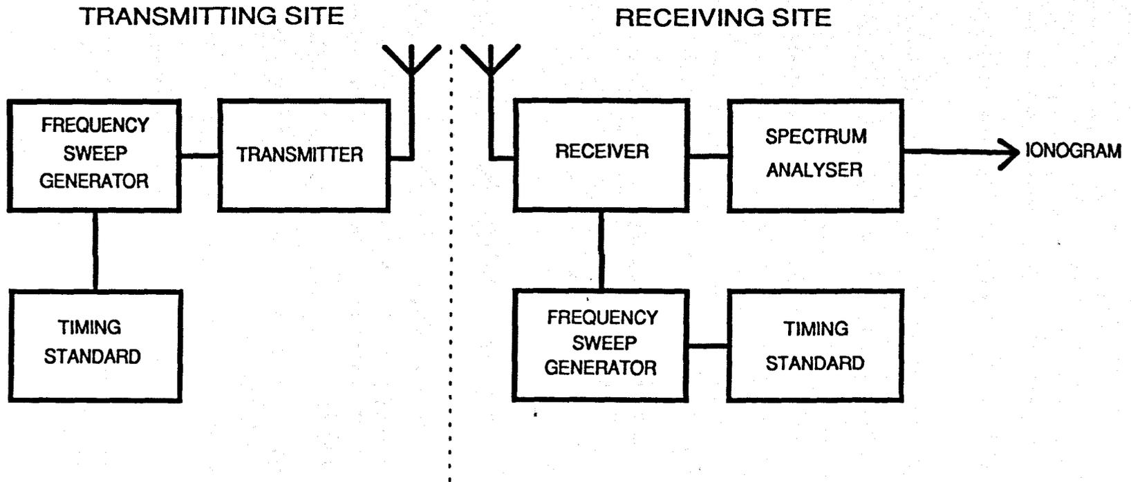
**FIGURE 7.4. PRINCIPLE OF CHIRPSOUNDING**
