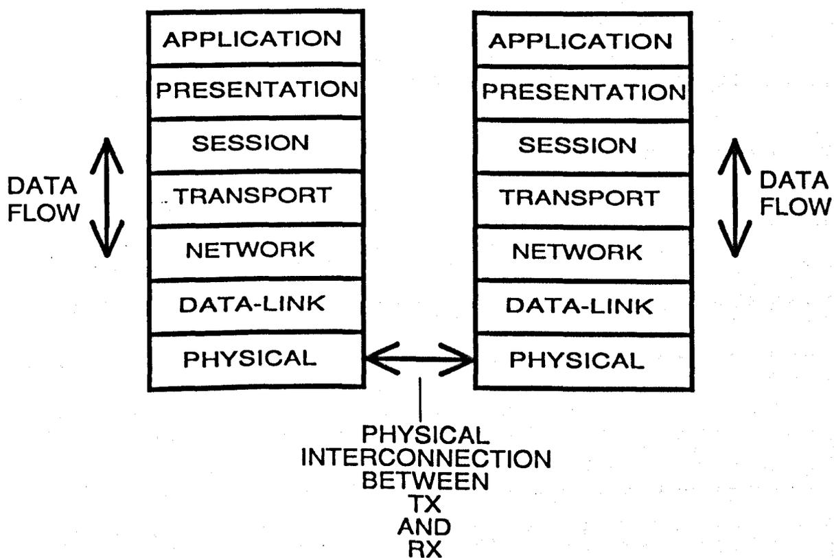
link set-up procedures, the provision of link management and link protocols.
