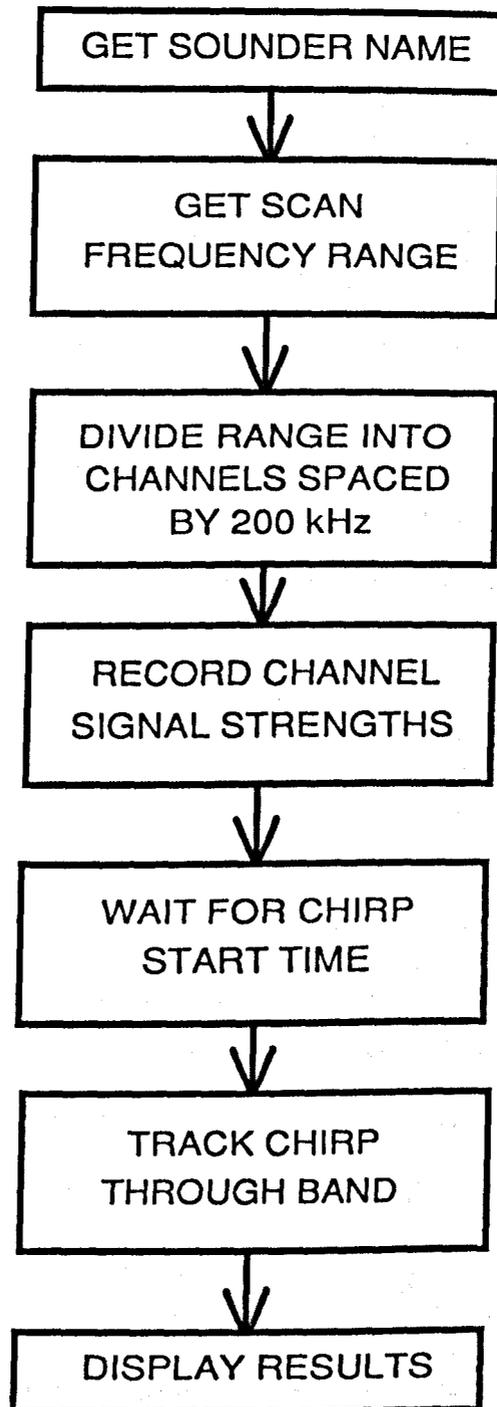
A block diagram of the estimator is shown in Figure 7.12. The hardware consists of a broadband HF antenna, an amateur grade HF receiver, an IBM pc XT clone, and a TMS 320C25 development board.
