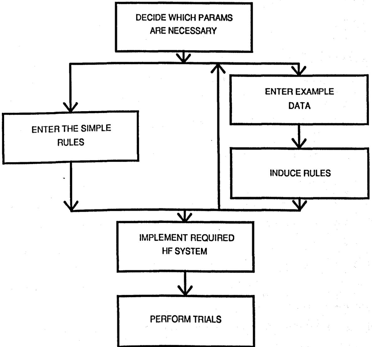
A design life-cycle showing how it is proposed to produce an HF communication system controller using inductive methods is shown in Figure 10.1.
