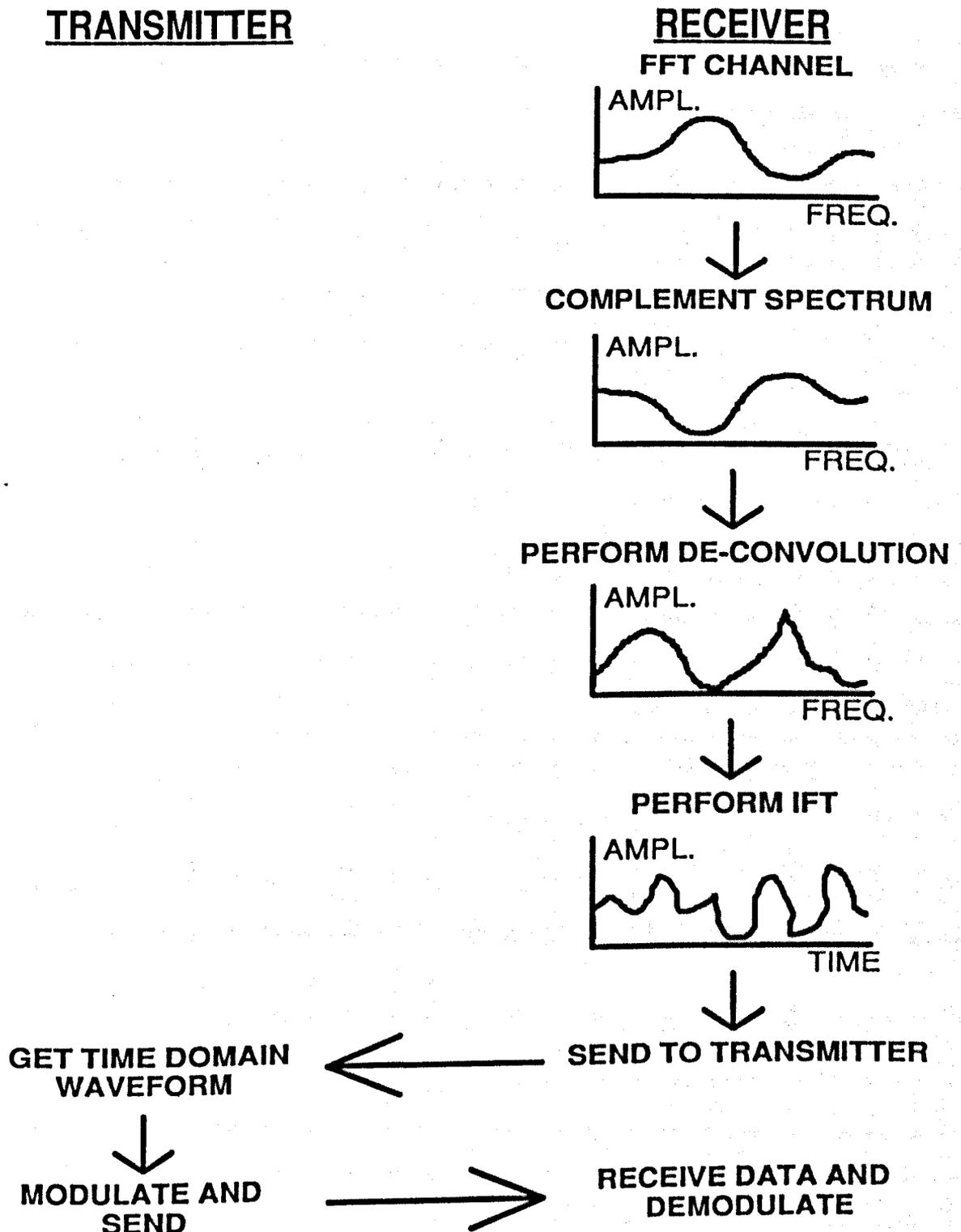
maximum information rate condition of equation 8.17. Advances in processor technology will allow a closer fit to the ideal case to be made, in real time. A technique which adapts the signal format of a transmission to match the prevailing noise/interference conditions more precisely than template correlation, termed spectrum complementing, has been conceived, the details of which are presented below.
