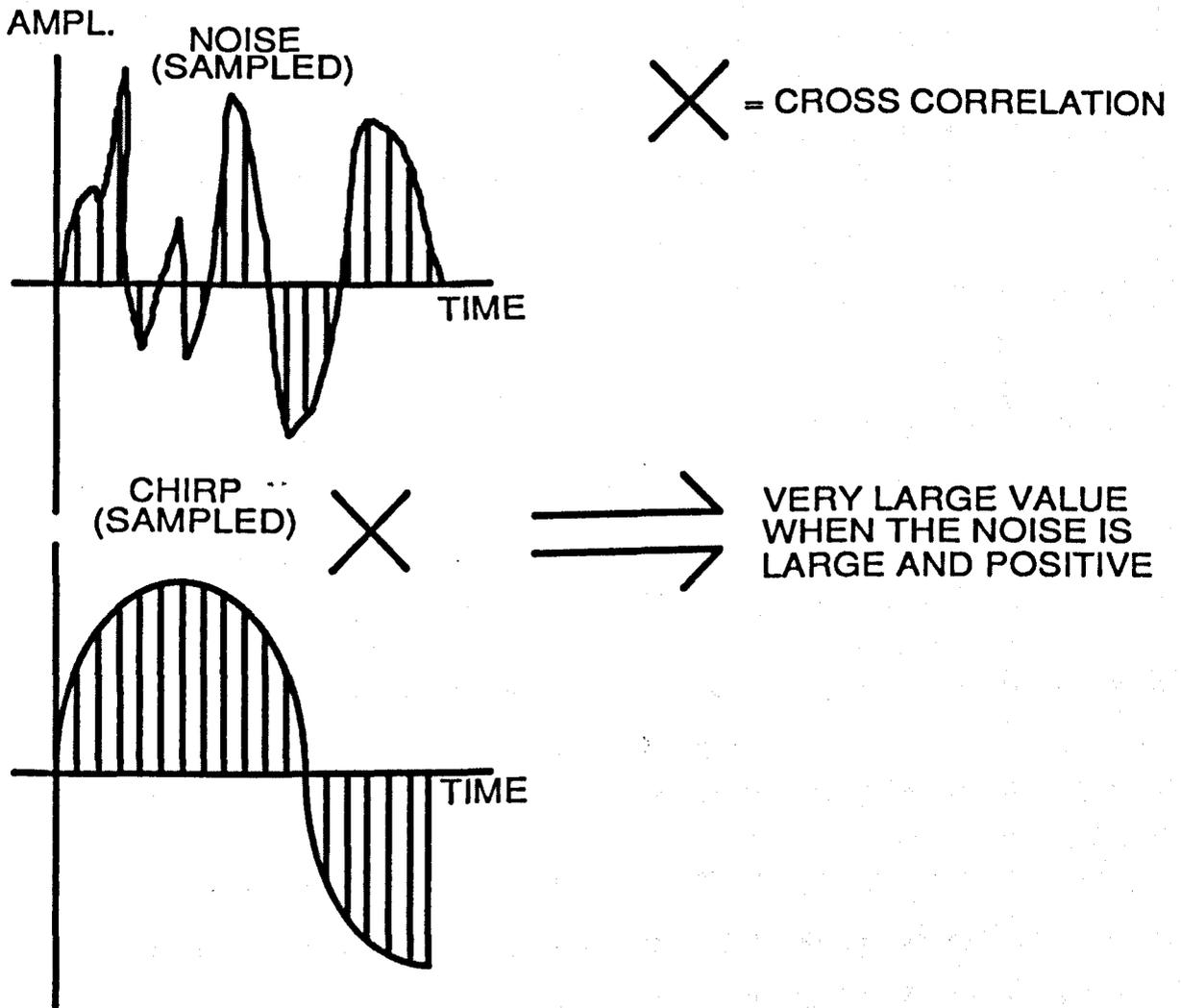
response of the filter due to the background noise from the receiver.
