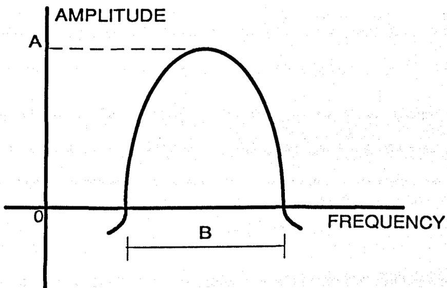
**FIGURE 8.5b. POWER SPECTRUM OF SINC(X) TONE**
