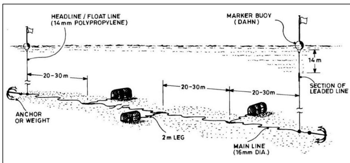
Figure 2.11: Schematic of the construction of a string of lobster pots deployed on the seabed. In the Holderness fishery, marker dans are replaced by inflatable buoys. Distances and specifics of the string construction in this survey are detailed above. Image provided from the Seafish database (Seafish, 2019b).
