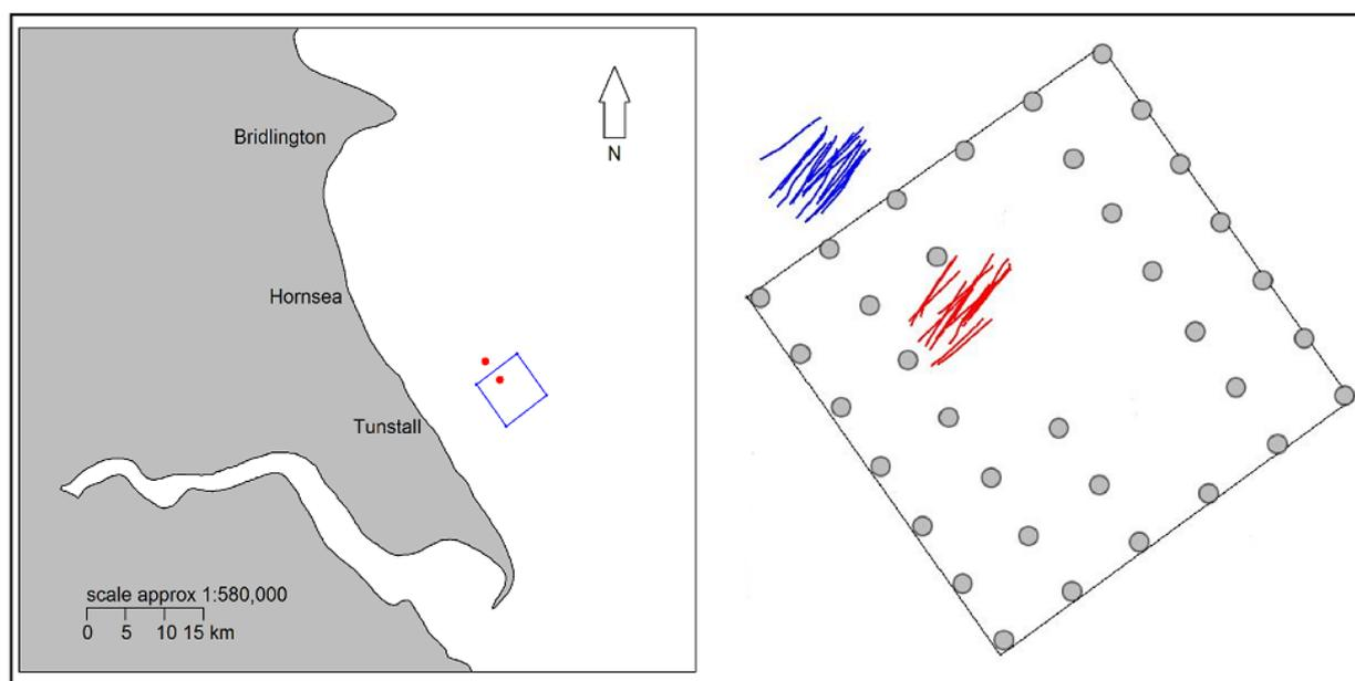
Figure 2.10: Location of the WMR OWF, the individual turbines marked and the locations of the control strings of pots to the North of the site and impact strings within the turbine array. The strings represent the sites where they are typically deployed, these strings are from the 2015 survey.
