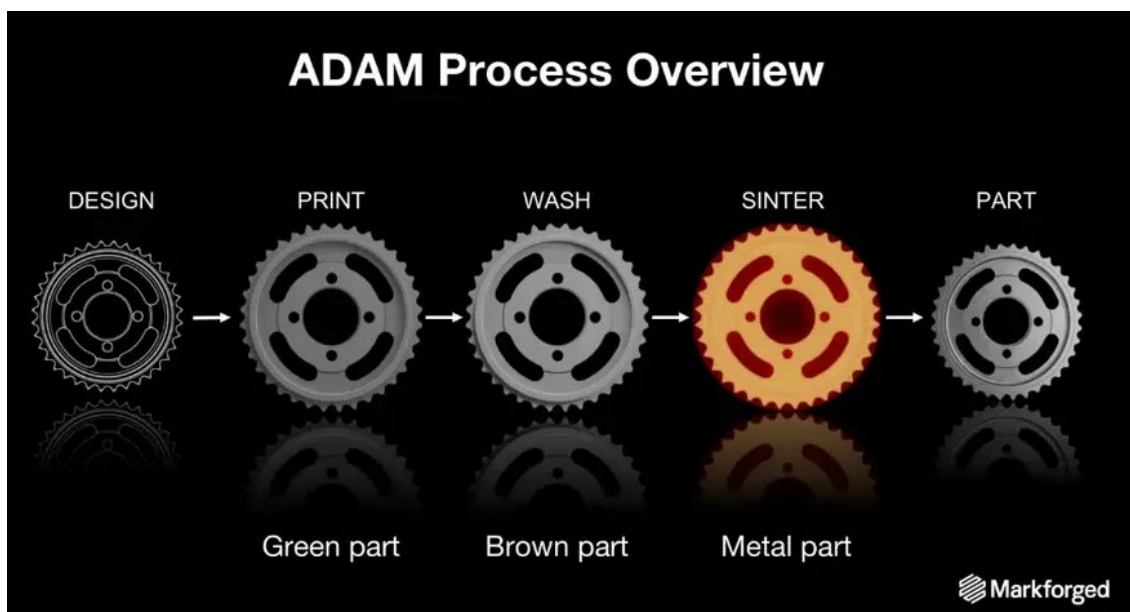
Figure 4.5: ADAM process of design, print, wash and sinter from Markforged. 5
