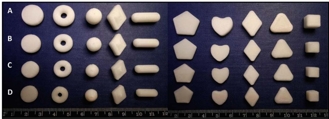
Figure 1.7: 3D printed paracetamol with different geometries. Reproduced with permission from Elsevier. 60
