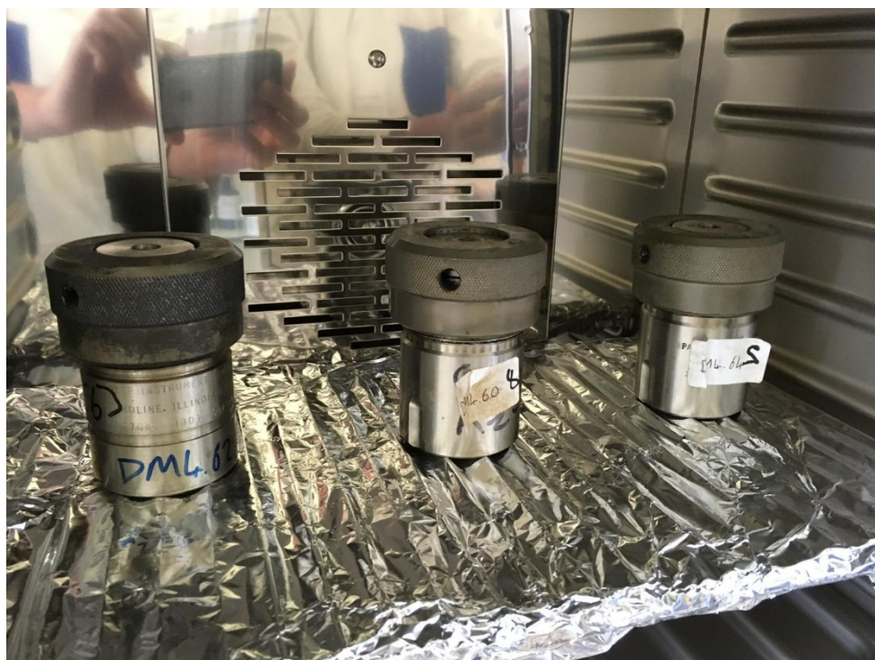
Figure 5.2: Autoclaves used for MOF-gel solvothermal synthesis.
