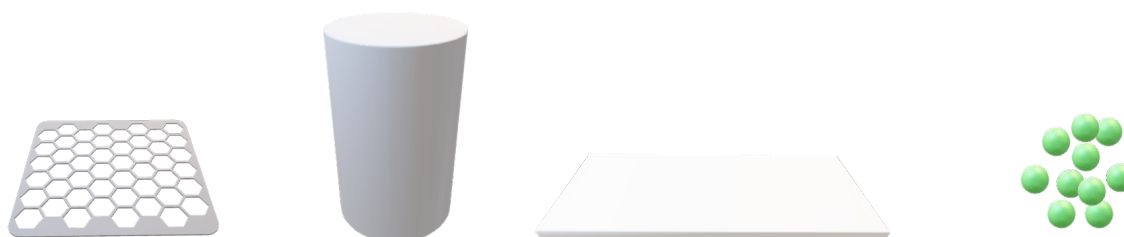
Figure 4.1: Honeycomb, cylindrical monolith, flat membrane and loose particles.
