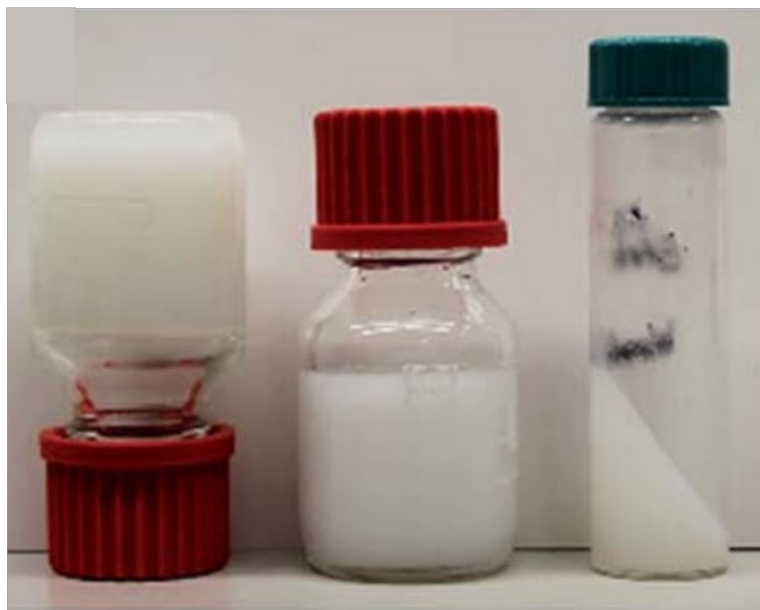
Figure 1.22: UiO-66 MOF-gel demonstrating the rheological properties by sample vial inversion. Reproduced under creative commons BY-NC 3.0 from Royal Society of Chemistry, 2017. 160
