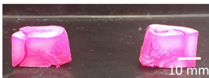
Figure 5.21: UiO-66 polymer monolith after a flow of rhodamine dye, sliced in half.
