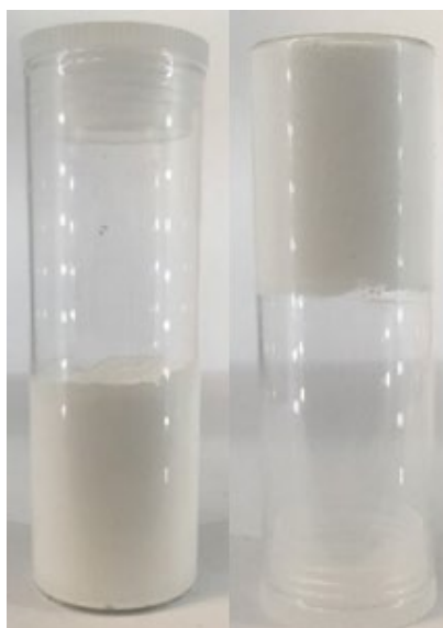
Figure 4.11: A rudimentary test of a sample vial upended containing UiO-66 in ethanol, demonstrating that the sample does not flow unless a shear force is applied.
