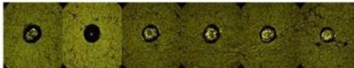
Figure 5.10. Irradiated spots on Graphene Oxide after 1000 Pulses at Different Fluences. 200x Magnification
