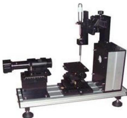
Figure 4.6 CAG 100 contact angle goniometer
