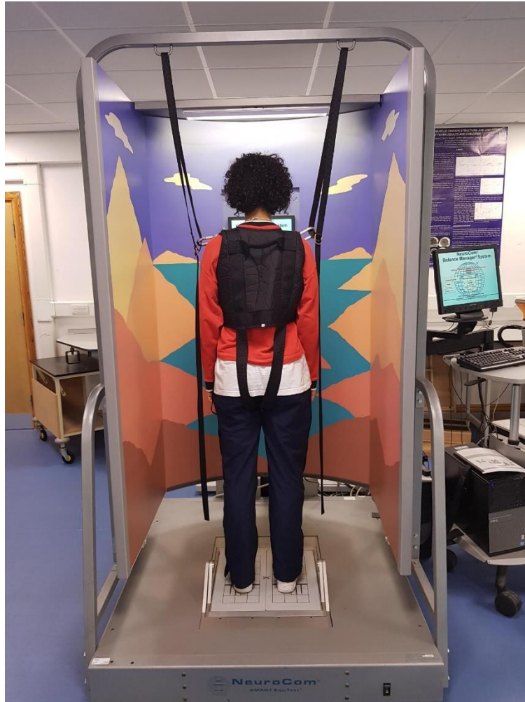
Figure 4.1. NeuroCom Smart Equitest system with sway-referenced moving visual surround and support surface. The participant is wearing a safety harness to prevent them from falling during the tests.
