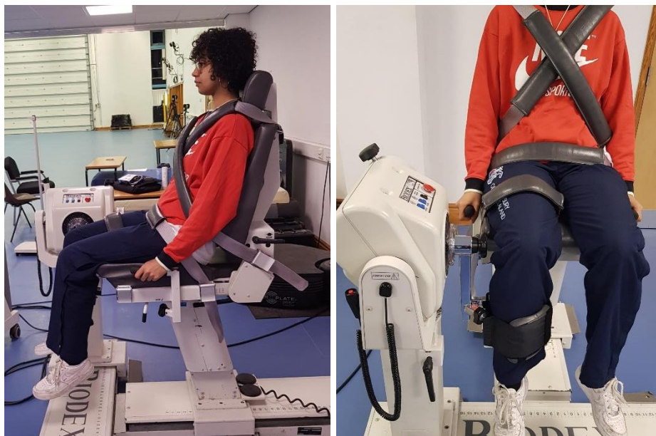
Figure 4.8. Isokinetic Dynamometer participant set-up with the right lateral femoral condyle aligned with the moving arm of the dynamometer. Image shows strappings across the chest, waist, upper leg and lower leg.
