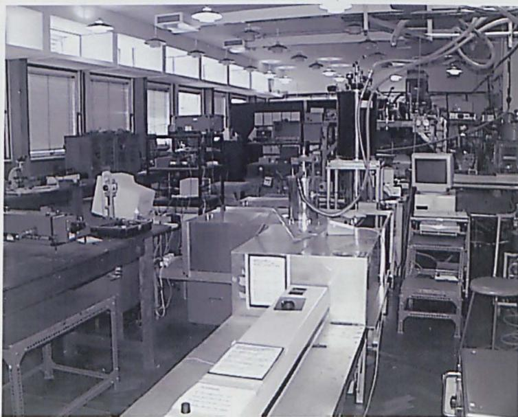
Figure 3.3:1: Photoluminescence spectroscopy laboratory,  $\text{Ar}^+$  laser pictured in the foreground and the liquid helium/nitrogen cryostat in the center.
