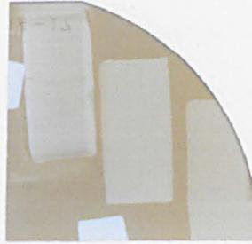
Figure 5.5:14 Nitrogen ion-implanted 6H-SiC quartered wafer laser annealed at 308 nm at  $1.5 \text{ J cm}^{-2}$  in air (left), and at 1.0 and  $0.9 \text{ J cm}^{-2}$  (centre and right respectively) at a pressure of 35 bar in argon: sample #6.
