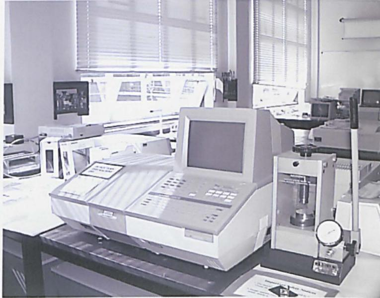
Figure 5.4:1 Fourier transform infrared spectrometer used in these experiments.
