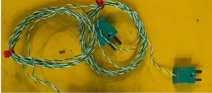
**Figure 4.13: K-type thermocouples used in experiment**
