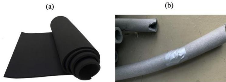
**Figure 4.10: Insulation material with (a) rubber and (b) foam**
