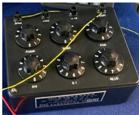
**Figure 4.9: Resistor box used in experiment**
