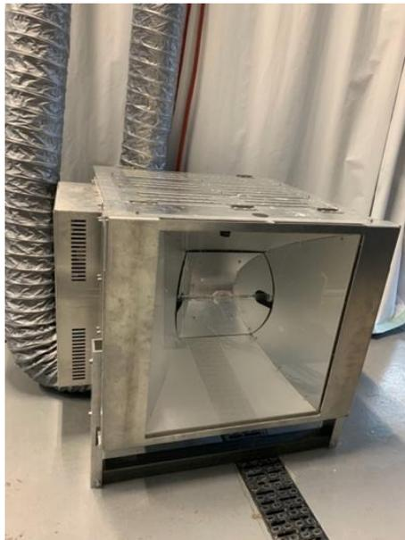
**Figure 4.4: Solar simulator used in experiment**
