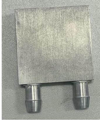
**Figure 4.6: Cooling block used in experiment**
