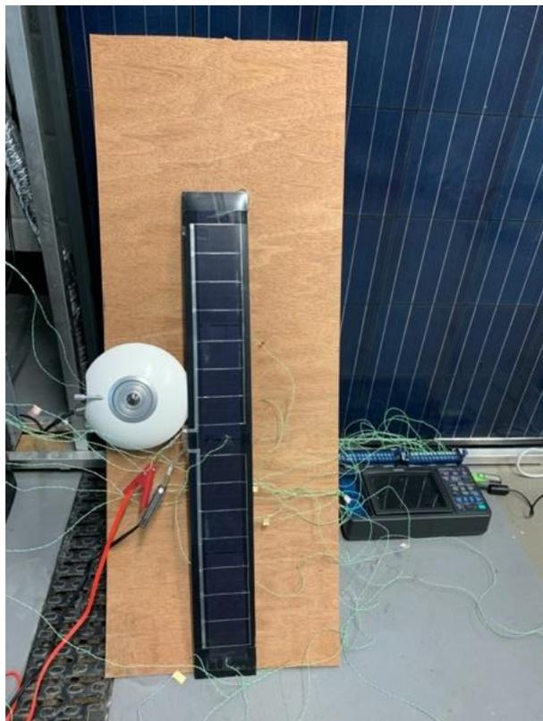
**Figure 4.22: Photovoltaic experimental setup**
