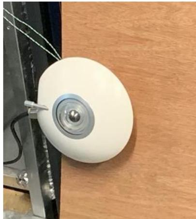
**Figure 4.12: Pyranometer used in experiment**
