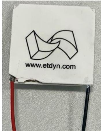
**Figure 4.3: Thermoelectric generator module used in experiment**
