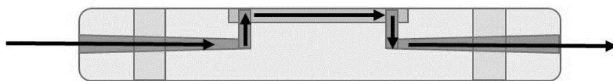
Figure 4.14 Direction of the fluid flow through the main PMMA body of microfluidic PCLS device A iteration one. Fluid flow depicted by arrows, tissue DMEM flows into device via inlet, passes over the tissue via the milled central chamber before flowing out via the outlet.
