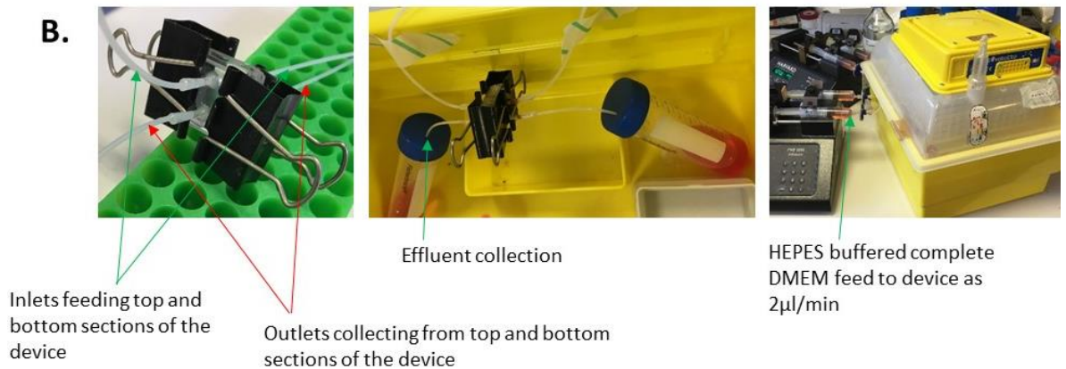
Figure 4.3 Microfluidic cell culture device one showing configuration of PDMS and PET membrane layers of the device during the process of seeding cell lines onto the membrane ( A ) and from left to right; the fully constructed device, the effluent collection arrangement and arrangement on infusion syringe pump ( B ).
