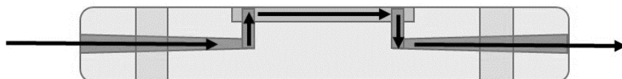
Figure 4.12 Direction of the fluid flow through the main PC body of optimised cell culture device. Fluid flow depicted by arrows, complete DMEM flows into device via inlet, passes over the PET membrane via the milled central chamber before flowing out via the outlet.
