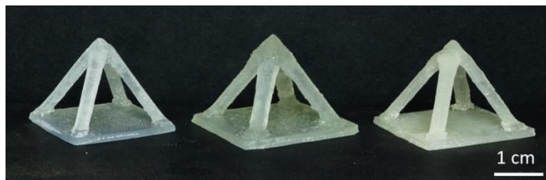
*Figure 55: 3D printed samples containing capsules with anisole cores, printed at 0, 5 and 10 wt% loading.*
