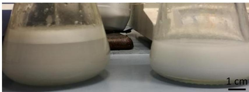
*Figure 62: (a) Filtrate obtained when epoxy was used as the encapsulated material. (b) Filtrate obtained when polyTHF was used as encapsulated material. This filtrate was found to be much milkier in appearance and which suggest that more polymer is present in the aqueous phase.*
