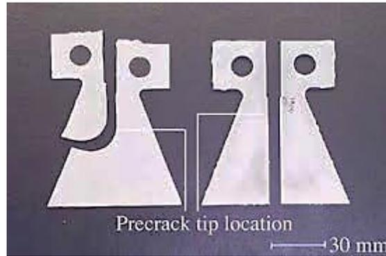
Figure 13: TDCB samples that have undergone loading tests to failure, showing the importance of the central groove for these specimens.<sup>99</sup> On the right is a sample without the 45° centre groove which shows deviation of the crack from the centre line. On the left is a sample with the centre groove which shows that crack propagation follows the centre line. The critical stress of the sample remained the same along the length of the crack for a certain length (between 20 and 40 cm).
