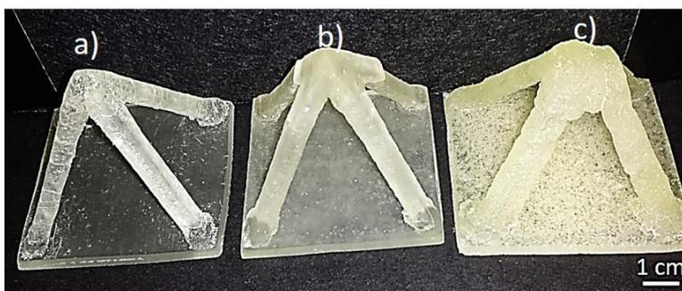
*Figure 88: 3D prints containing various capsule loadings. a) No capsules, b) 15 wt% epoxy capsules and c) 15 wt% EPA UF capsules. Despite both capsule containing prints having a 15 wt% loading, the appearance of the print containing the epoxy capsules is much closer to the non-loaded print.*
