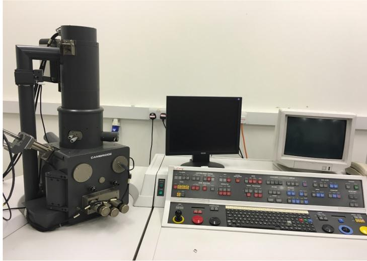
Figure A-A4 Scanning electron microscope (SEM) stereoscan 360
