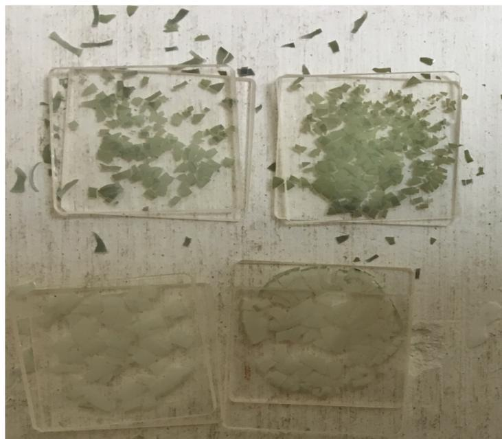
Figure A-A9 Broken AAO membrane during calcine process
