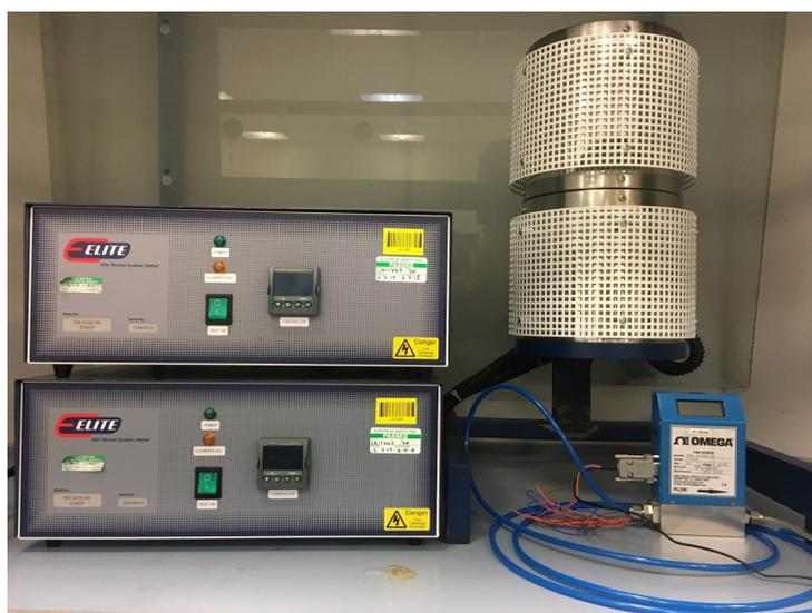
Figure A-A3 Two-stage catalytic-pyrolysis reaction system
