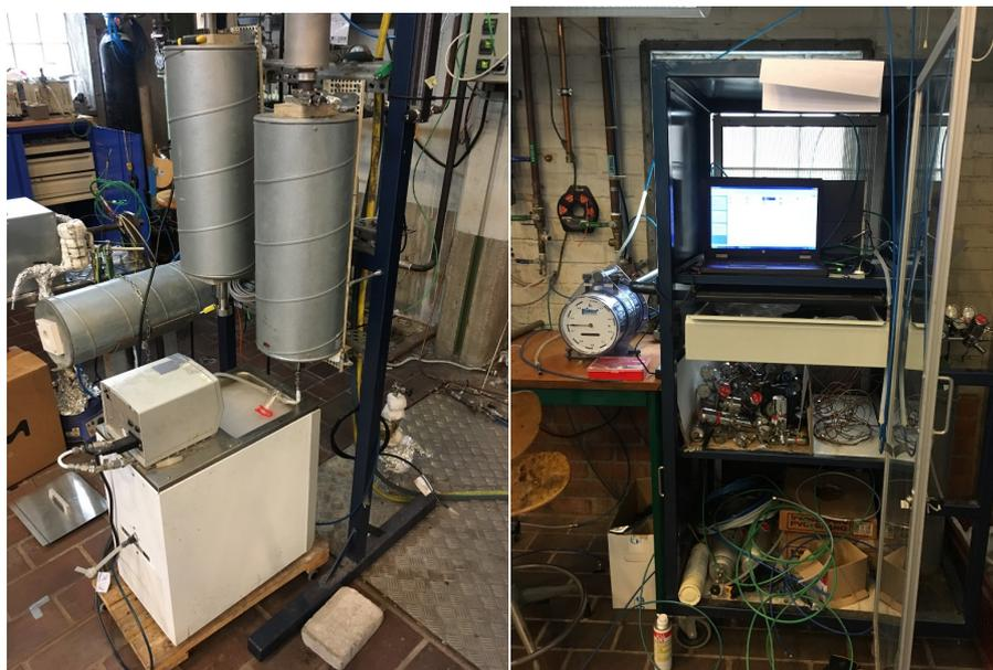
Figure A-E7 Catalytic pyrolysis of plastics with online GC
