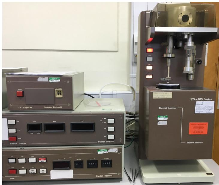
Figure A-A7 Thermogravimetric analyser (TGA) STA-780 Series
