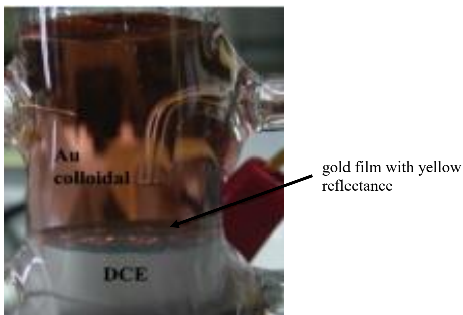
Figure 19. Gold film with yellow reflectance forming from citrate-coated gold nanoparticles, at a water and 1,2-dichloroethane interface. From the work of Younan et al. 81 .
