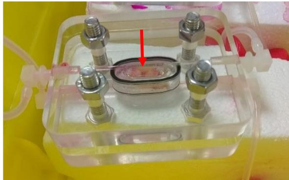
*Figure 6.5 Gen2.T1 chip set up with gut tissue, the red arrow highlights the location of the tissue.*
