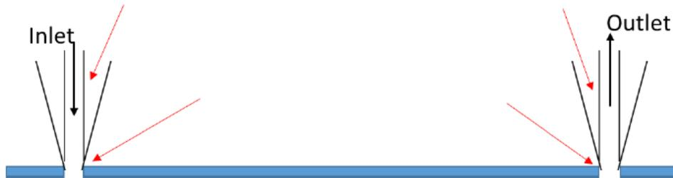
*Figure 3.6 Schematic of the glass outer chip layer of the dual channel chip. The tubing connectors (made from pipette tips cut to size) are the most likely section of the chip to leak. This can occur in two ways: firstly, through the connection between the pipette tip and the glass, and secondly between the connection of the pipette tip and the tubing.*
