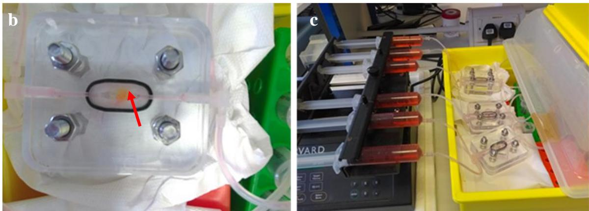
Figure 6.3 Photograph of chip set up for sample gut001. a) Flow chart illustrating the processing of tissue sample gut001. B) Photograph of the chip set up with gen2.3 carrier and gut tissue biopsy indicated with a red arrow. c) Set up of three chips in an incubator.
