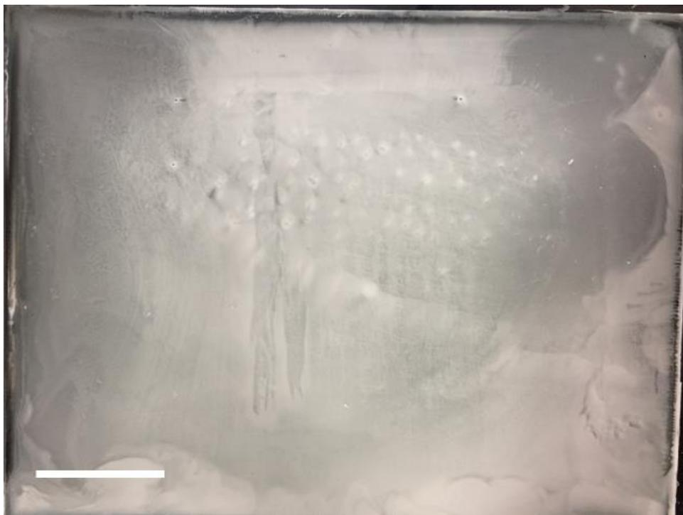
**Figure 3.20** Bioimprint produced by exposing curable PDMS to a layer of fixed yeast cells deposited on functionalised glass slides from aqueous glucose solutions. The dimensions of the bioimprints are 2 cm × 2 cm. Scale bar represents 5 cm.
