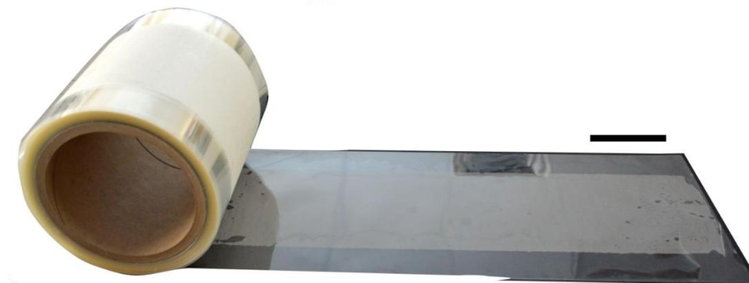
**Figure 3.37** Photograph of the replica HL60 bioimprints augmented to cover  $0.4 \text{ m} \times 100 \text{ m}$  by R2RNIL. Scale bar represents 20 cm.
