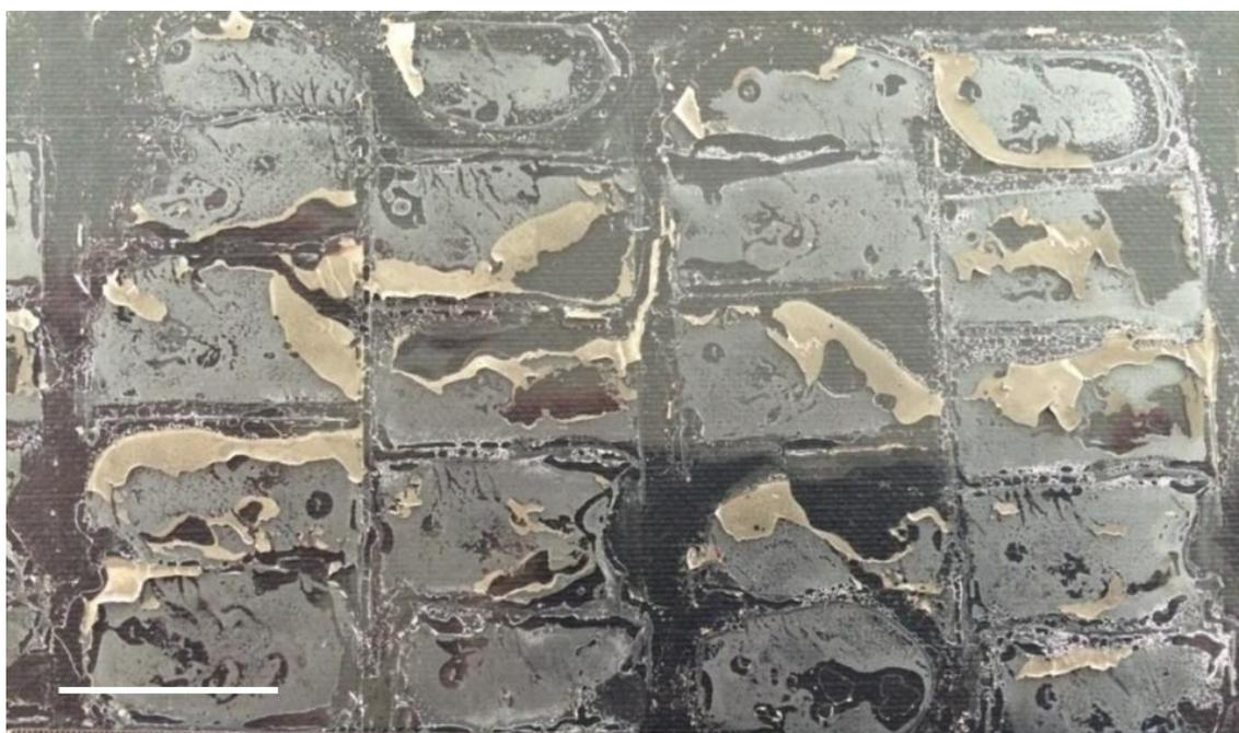
**Figure 3.33** Photograph of a patchwork of multiple positive imprints made sequentially next to the previous one yielding a total imprinted area of 15 cm × 5 cm. Image taken after use in R2RNIL device; deterioration of metal coating is clearly visible. Scale bar represents 2 cm.
