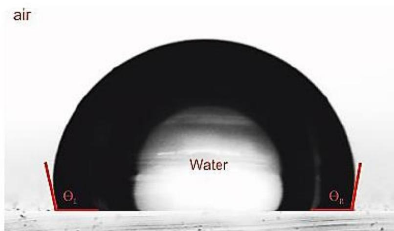
**Figure 2.5** Contact angle measurement of a sessile drop of MilliQ water on PDMS substrates.
