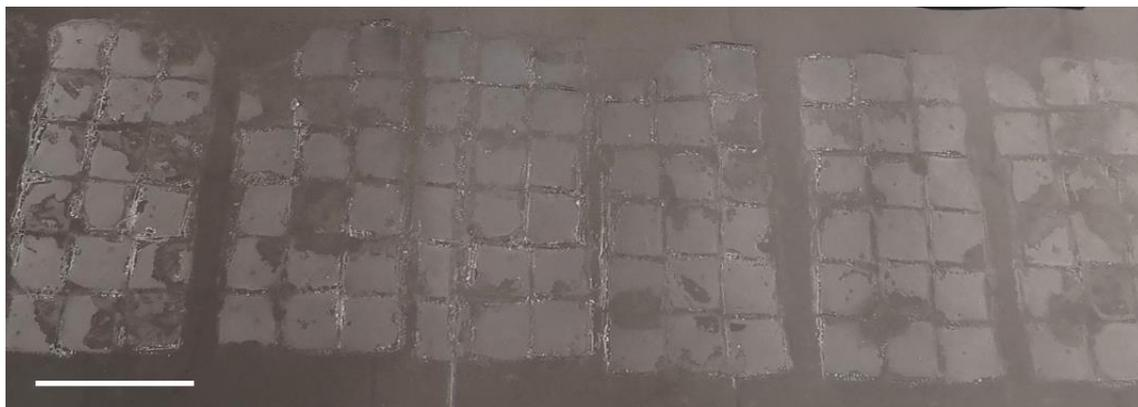
**Figure 3.34** Photograph of replica bioimprint embossed into UV curable PU photoresist R2RNIL from bioimprints made using Jurkat cells deposited by via the Cytospin centrifuge. Scale bar represents 6 cm.
