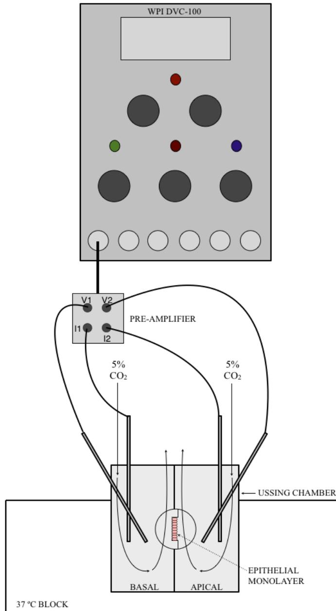
**Figure 3-3** — A schematic depiction of the DVC-100 V/I clamp apparatus showing a BOEC-filled Snapwell™ sandwiched within a gassed and temperature controlled Ussing chamber. Probes protruding from the DVC preamplifier were inserted into the chamber to enable voltage manipulation and current measurements
