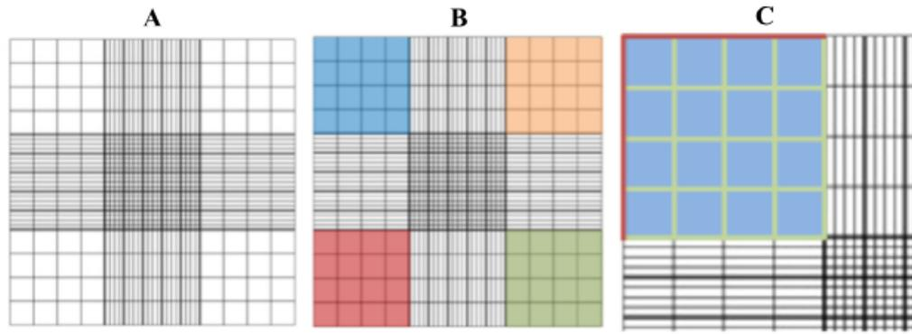
**Figure 2-1** — **A:** Image of of the complete haemocytometer at x20 magnification. **B:** Cells were counted within the four corner sections of the haemocytometer highlighted in blue, orange, green and red. **C:** Any cells present on the outer red lines were excluded from the count whereas cells within or verging on the boundaries highlighted in green were suitable for inclusion. To perform a viability assay the following formula was used:
