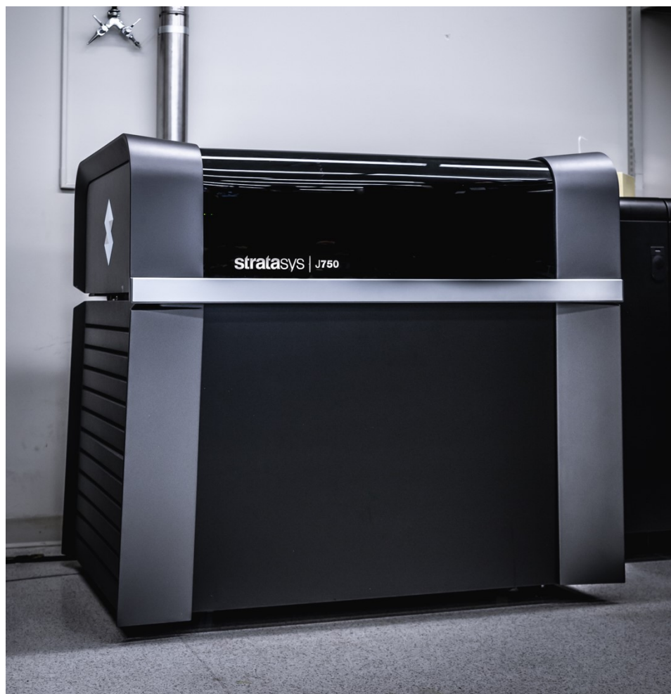
Figure 2.3: Stratasys J750 Digital Anatomy Polyjet printer used for congenital heart models for surgical simulation and anatomical models (Stratasys, Eden Prairie, MN).
