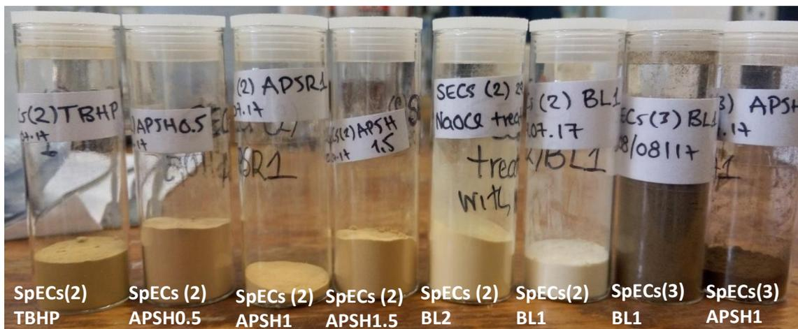
**Figure 32:** Modified SpECs. The bleaching procedure on SpECs(2) changes the SpECs colour from yellow to white (6<sup>th</sup> vial counting from left to right). For SpECs(3) it changes the colour from dark brown to lighter brown (7<sup>th</sup> vial).
