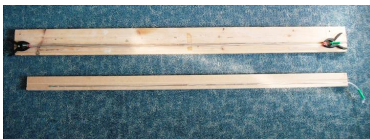
Figure 4: Left: initial frame with clamp to secure tube. Right: final frame which holds tube securely along entire length
