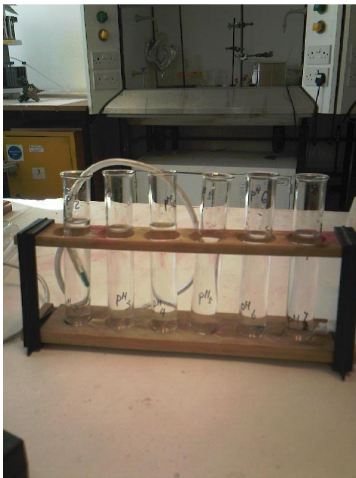
Figure 10: Test tubes containing pH solutions of different acidity with distal tip of nasogastric tube in situ
