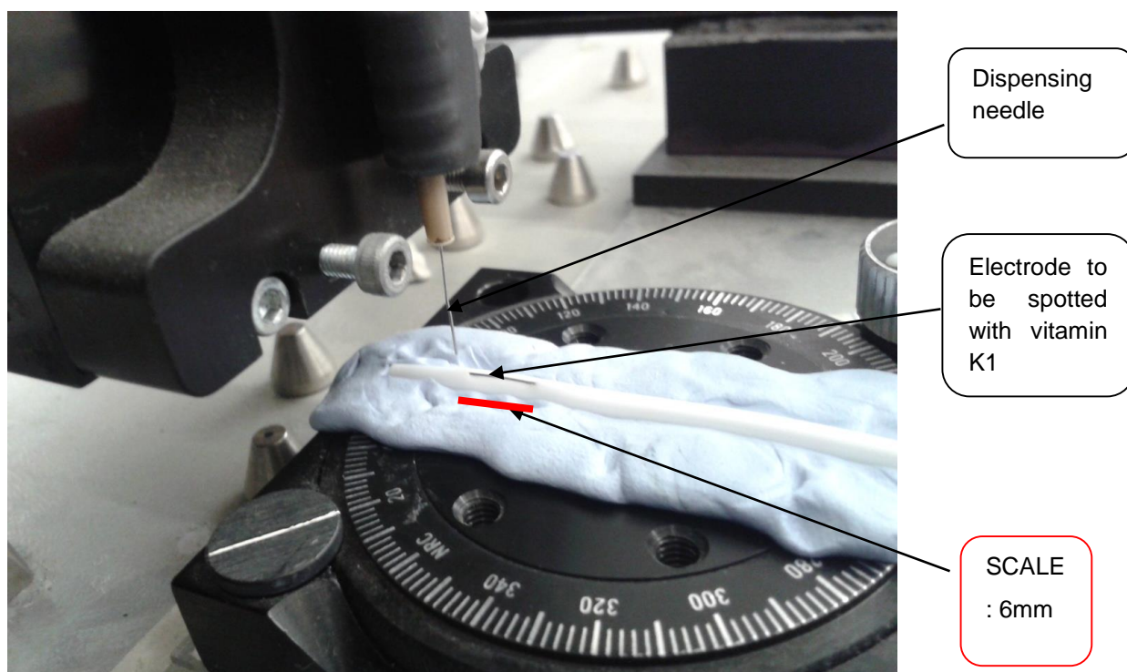
Figure 16: Dispensing needle applying micro spots of vitamin K1 to electrode surface
