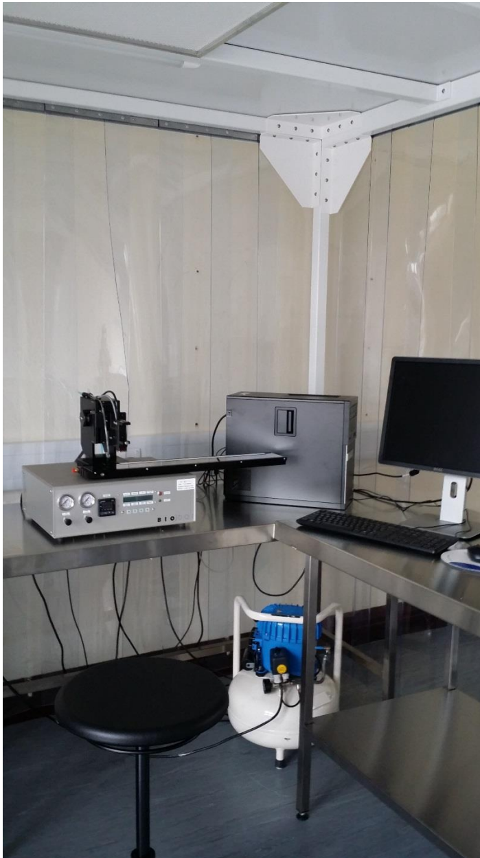
Figure 23: Validated cleanroom with Biodot machines installed for application of sensing materials
