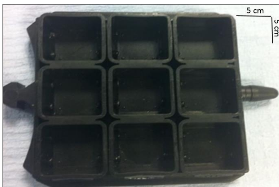
Figure 2-3: An array biochip array holder (RANDOX), which is capable of multiple detections on glass slides and plastic slides, cell holder was aligned under the CCD camera inside the box for CL detection.
