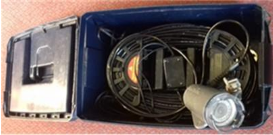
Figure 3-2. Drop-down video camera used for capturing point transect video footages
