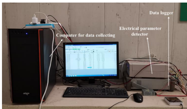
Fig. 5-15 Data collecting devices for the heat pump experiment
