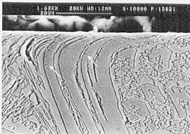
b) Cracking of large carbides
