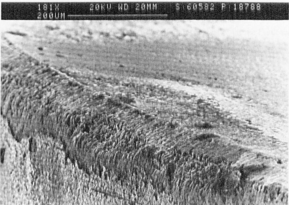
**Figure 6.12** General view of the cutting edge showing chipping developed over the cutting edge (1 minute, S65m/min, F0.25mm/rev, DOC0.65mm).
