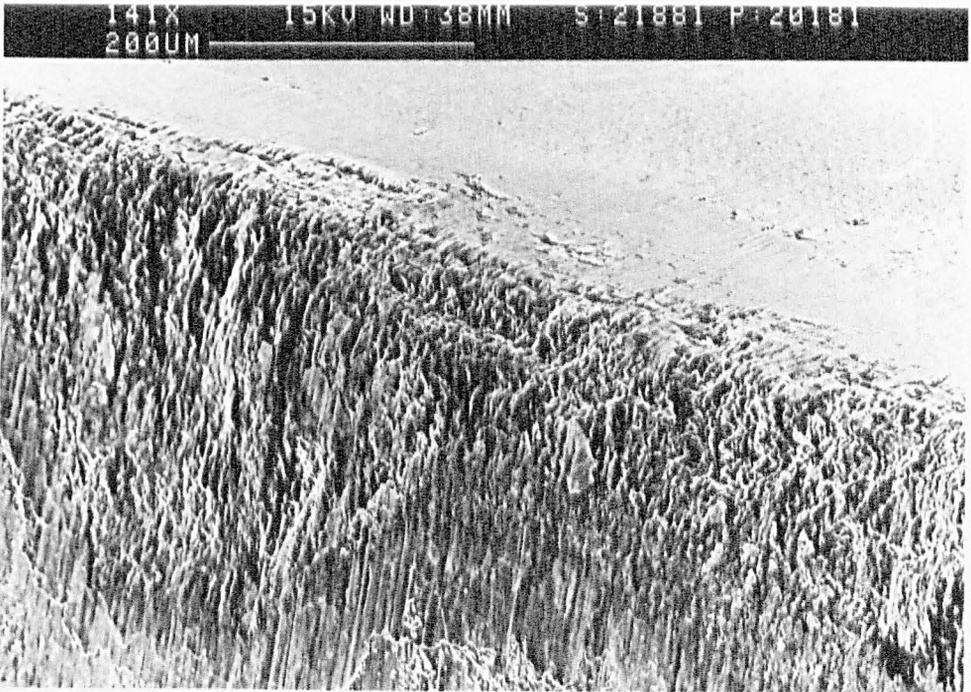
**Figure 6.19** Tool wear when machining Hardfacing B at higher speed (85m/min.) showing severe damage of the cutting edge and the flank of the tool (F0.25mm/rev, DOC0.65mm).
