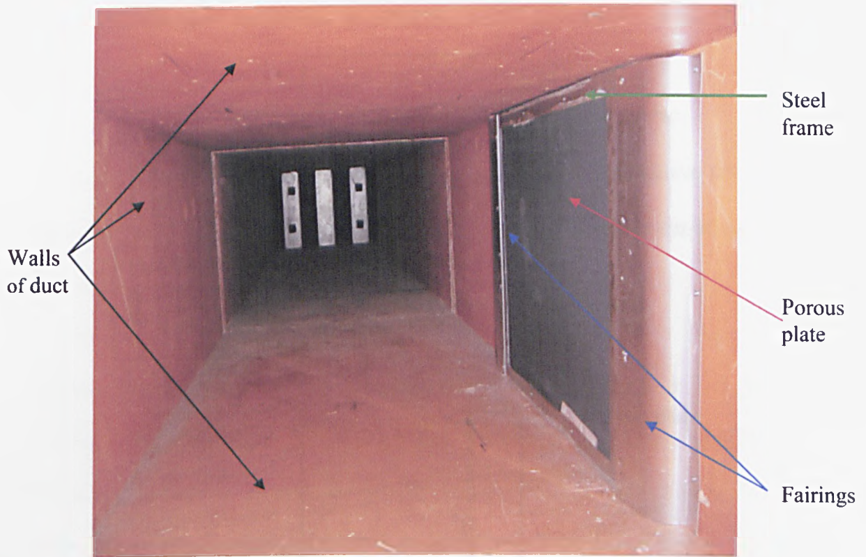
Figure5.2: Picture of the porous plate mounted on side of the duct wall.
