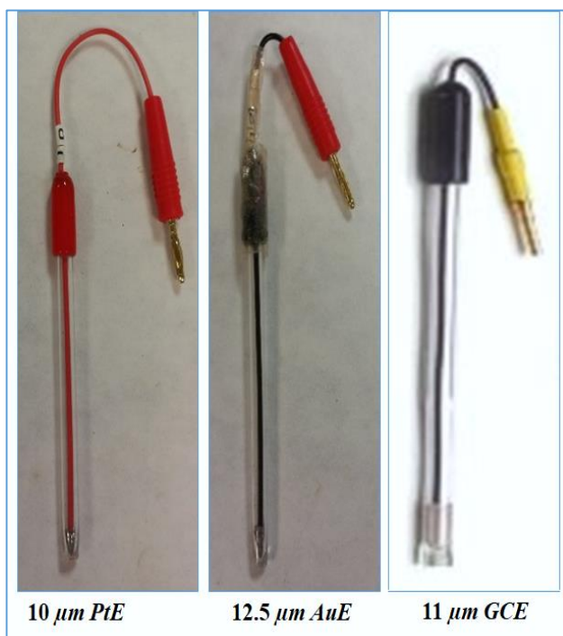
Figure 7.4: Microelectrodes; Platinum (Pt), gold (Au) and glassy carbon (GC)
