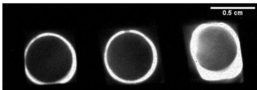
Figure 4.13. Represent the signal after the addition of artificial saliva spiked with cortisol standard solution 10 \text{ ng ml}^{-1} . The signal was decreased due to the reaction between the antibody and antigen that restrict the Fc moiety from its role as an oxidising agent for luminol and hydrogen peroxide reaction. The scale bar is 0.5 cm.
