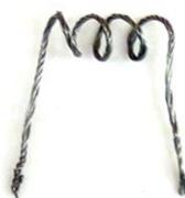
Figure 2.4: *The shape of molybdenum filament consisting of seven strands of Mo metal.*
