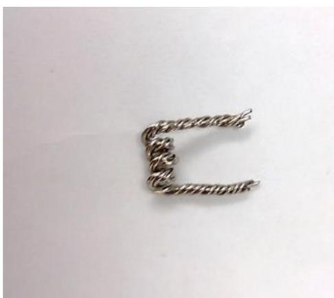
Figure 2.2: Nickel filament consisting of five strands of Ni metal
