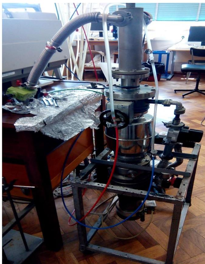
Figure 2.7: *An Edwards Diffstak 100 vapour diffusion pump and liquid nitrogen trap.*
