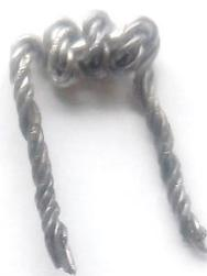
Figure 2.3: *Cobalt filament consisting of five strands of Ta metal wound around a Co rod.*
