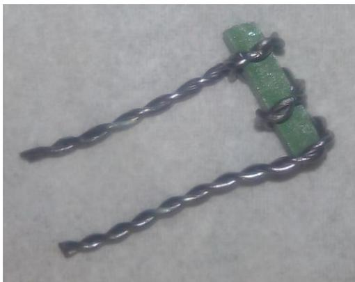
Figure 2.5: *The shape of chromium filament and a tantalum support consisting of two strands of Ta metal wound around a Cr bar.*
