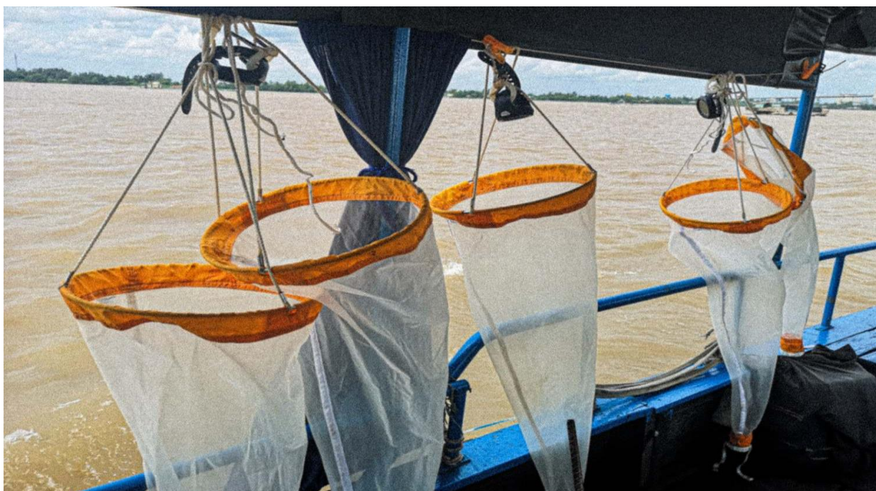
Figure 3.8: Plankton nets used for sampling microplastics in the Mekong River.
