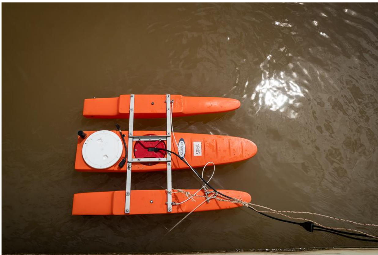
Figure 3.7: ADCP used to record and calculate flow of the river.
