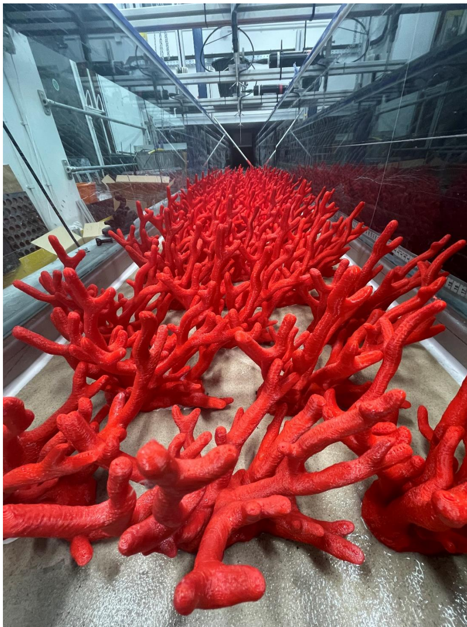
Figure 3.13: The flume setup of the dense coral canopy
