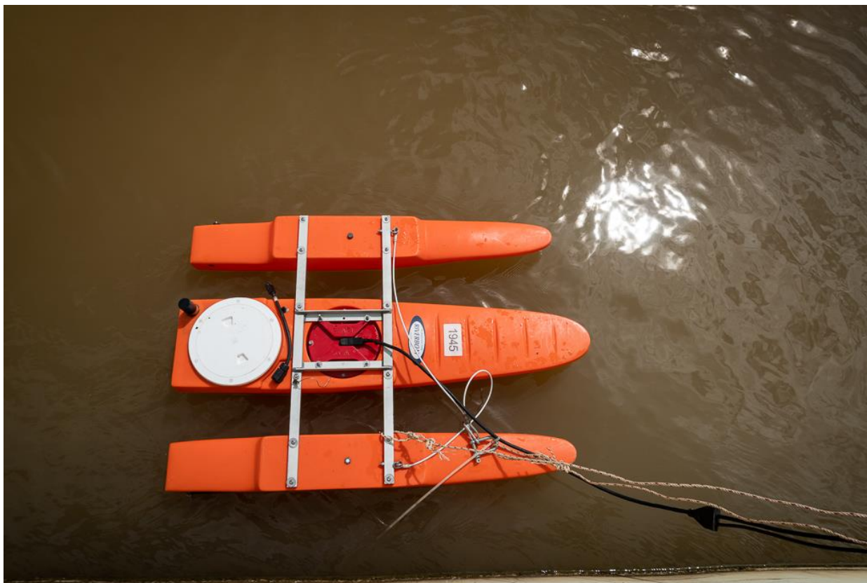
Figure 5.12 ADCP used to record and calculate flow of the river.
