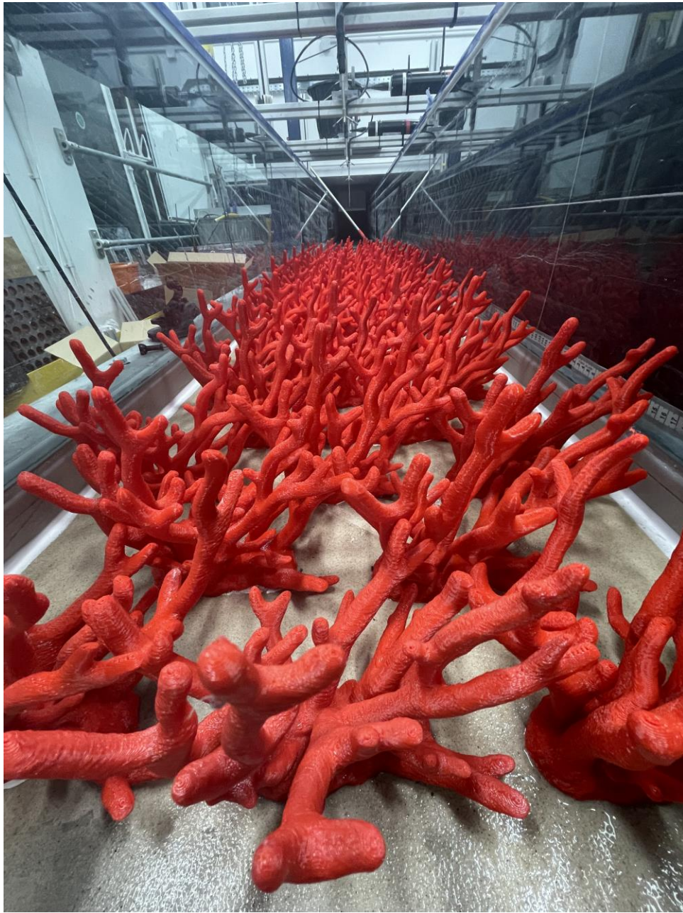
Figure 6.4: The flume setup of the dense coral canopy
