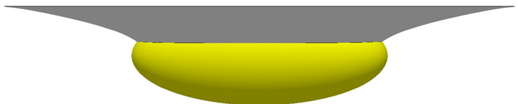
Figure 4-5 Interfacial deformation calculated from Surface Evolver for an ellipsoid with m = 2.6 , \phi = \pi/2 , h = -h_c for contact angle (a) \theta_w = 45^\circ and (b) \theta_w = 90^\circ .
