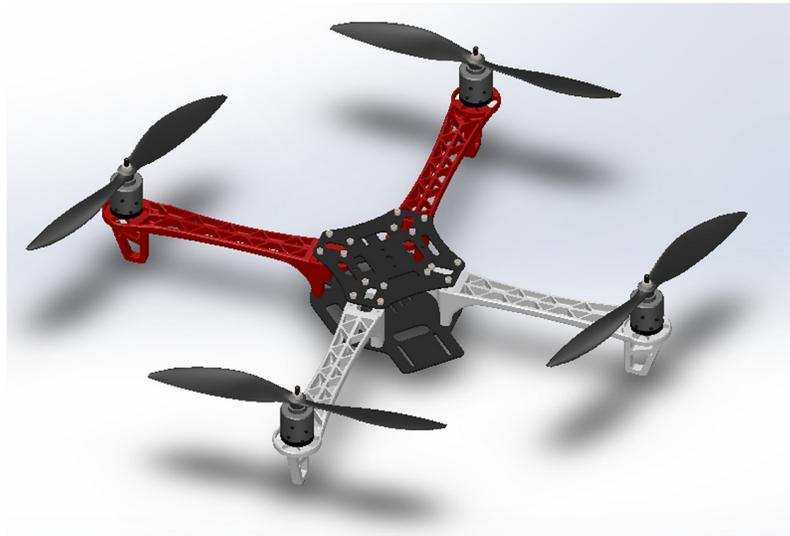
**Fig 10. Quadrotor's 3D CAD model.**
