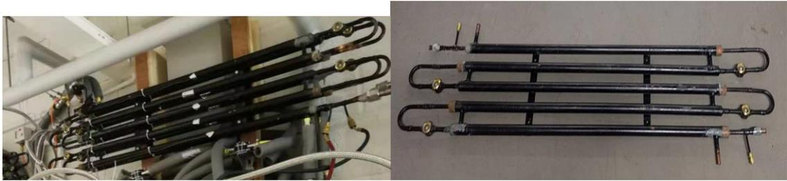
**Fig.5-3.** A photograph of such a co-axial condensation heat exchanger
