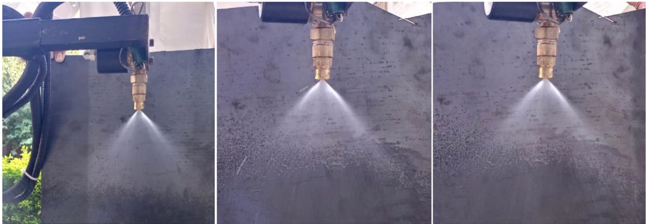
Fig 11. Constant spray angle achieved under different number of active solenoid valves at constant pressure.
