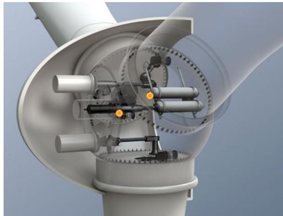
Figure 1.9: Hydraulic pitch system of wind turbine system (from google images)
