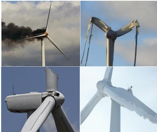
Figure 1.2: Different wind turbine blade failures (from google images).
