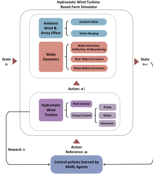
Fig. 3. Sub-model hierarchy of the HWT-based farm simulator for MARL. Note that we only illustrate one turbine in this figure for convenience. In fact, this simulator can include multiple turbines during operation.
